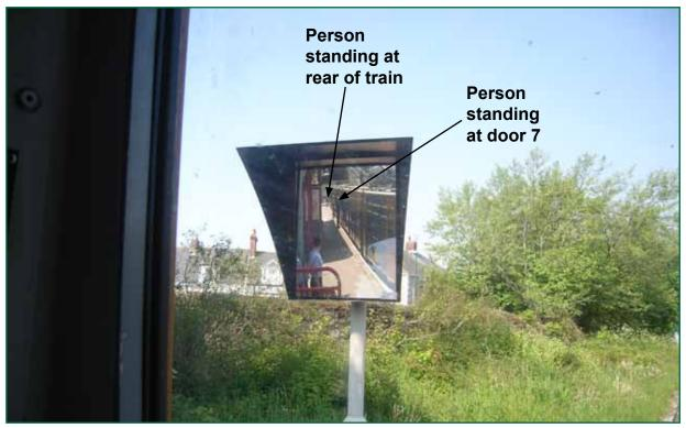
Figure 9: Typical view of the platform/train interface from the driver's cab through the mirror on platform 2 at Jarrow station (Note that the station canopy shadow at the time of the incident would not have been so pronounced)
