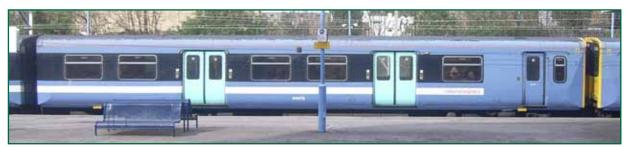
Figure 6: Class 315 EMU with doors at 1/3 and 2/3 positions.
