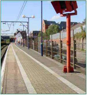
Figure 14: Eight-car monitor position in October 2001. The head of the DOO monitor is rotated to the left and not an at angle to the platform edge (photograph courtesy of Network Rail)
