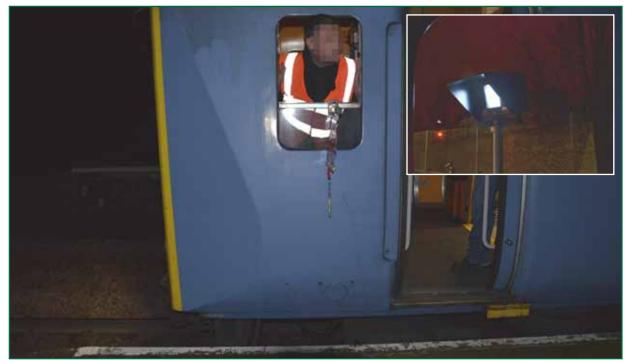
Figure 13: View of DOO CCTV monitor from train drivers stopping position on the night of the accident.
