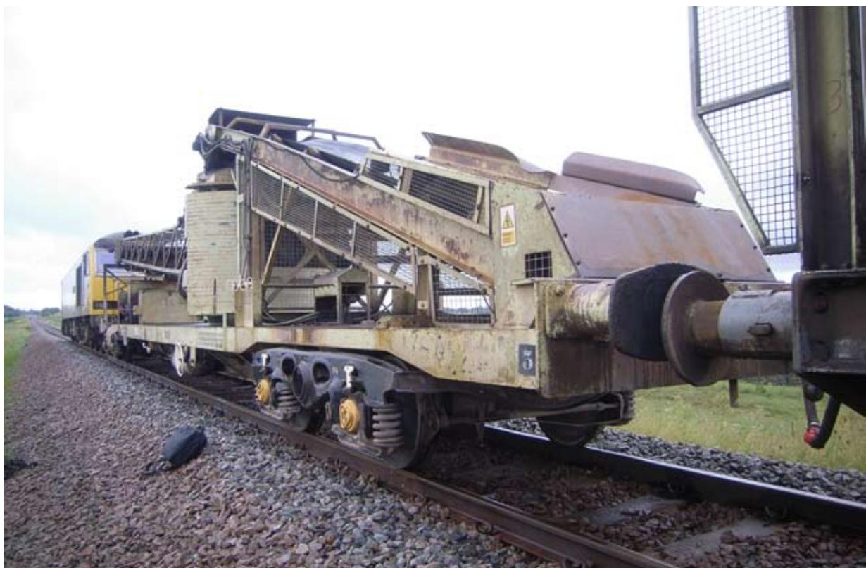
Figure 5: Self-discharge train incorporating the off-load wagon showing the conveyor belt arrangement
