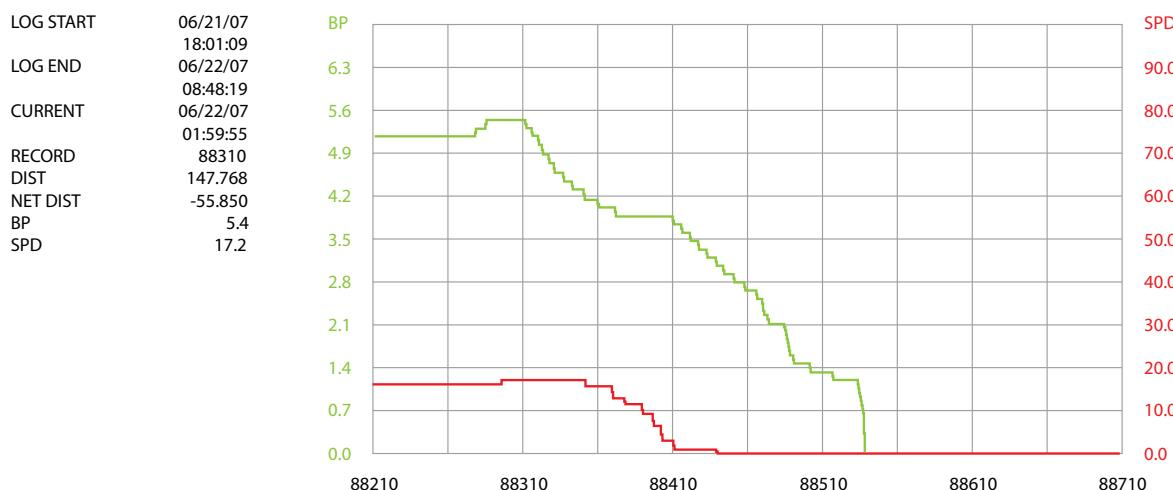
Figure 30: Locomotive 60068 OTDR reading of speed (red trace) and brakepipe pressure (green trace) at 01:59:55 seconds 22 June 2007
