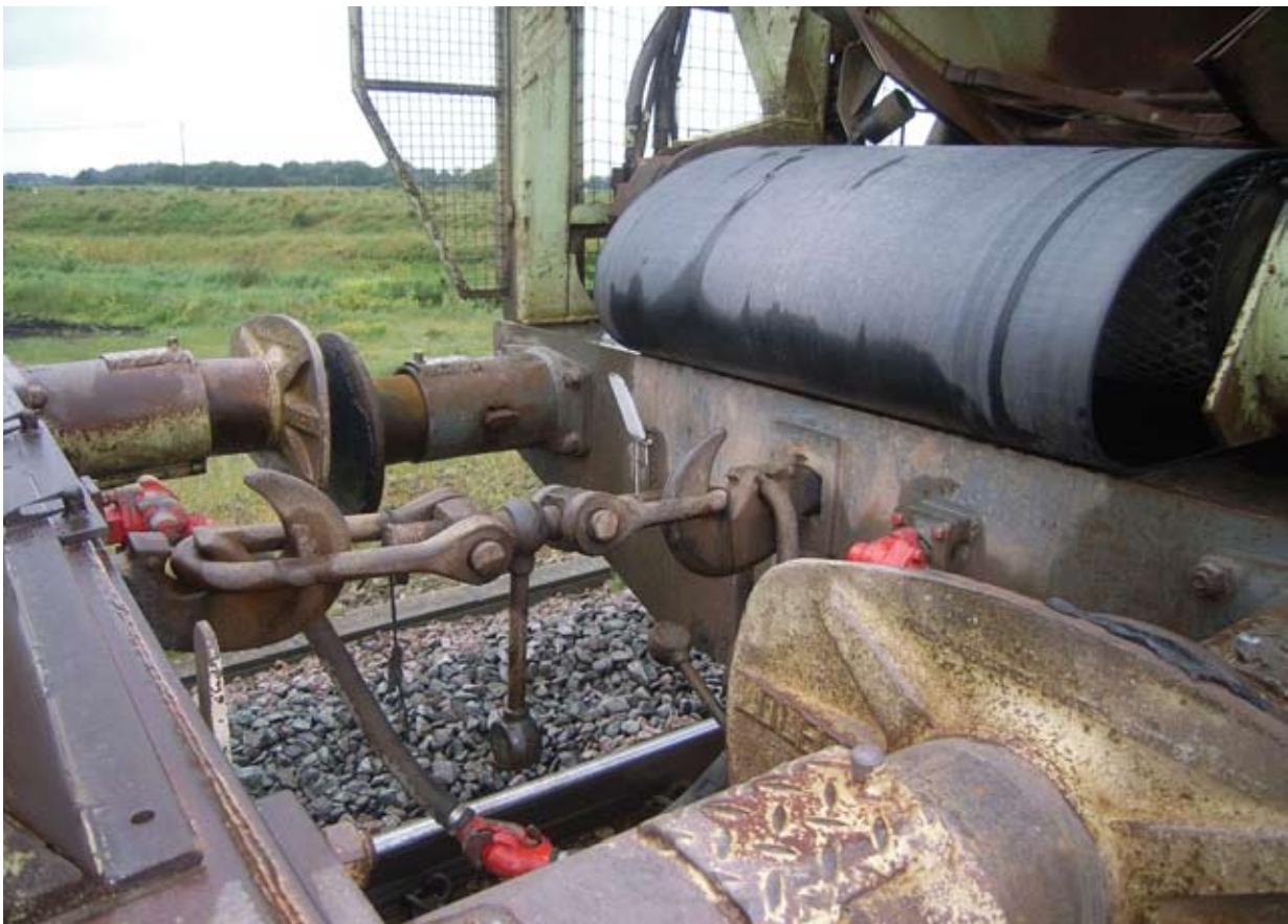
Figure 4: REDA coupling arrangement
