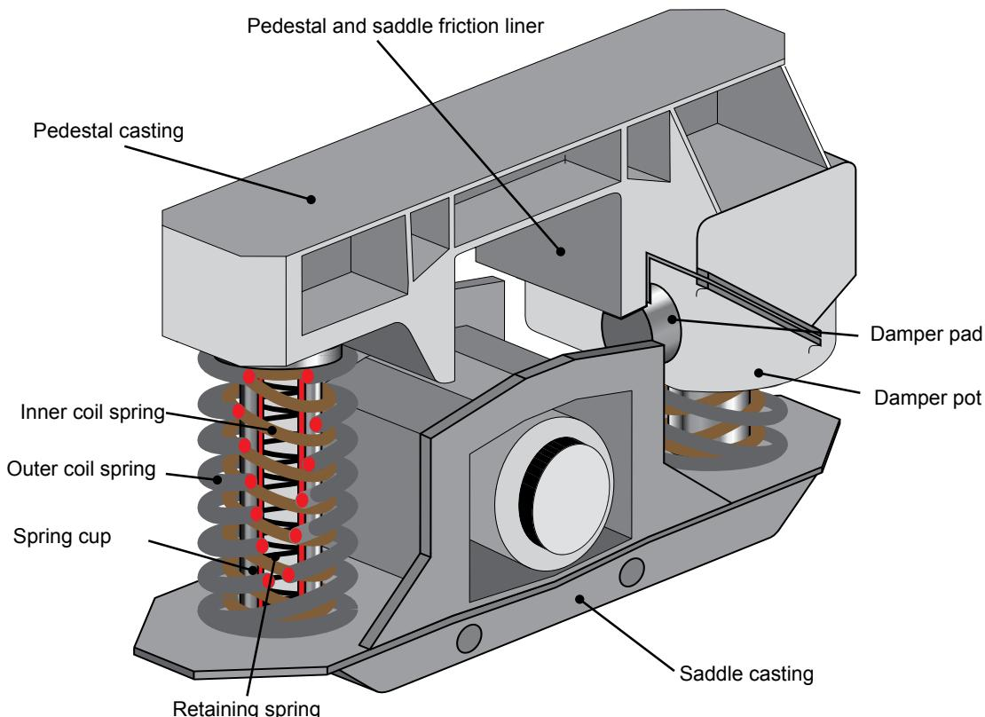
Figure 40: Diagram of GFA suspension and components
