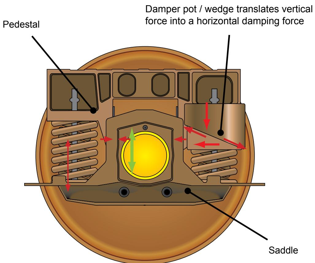
Figures 7: GFA suspension showing damping forces of pedestal and saddle
