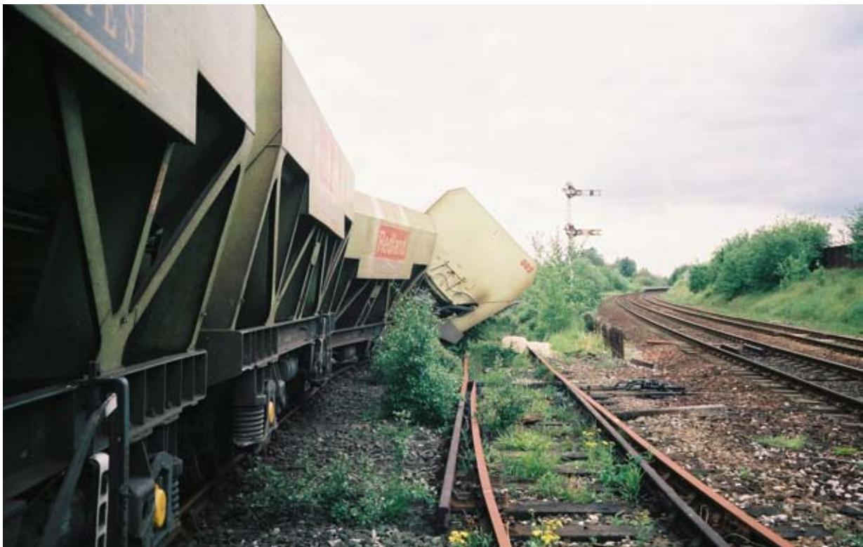
Figure 44: Image showing derailed wagon REDA 16002
