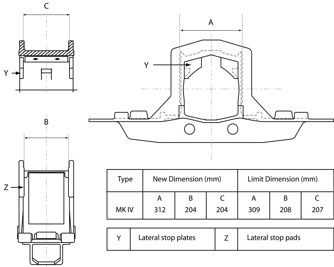
Figure 53: Saddle casting and tolerances
