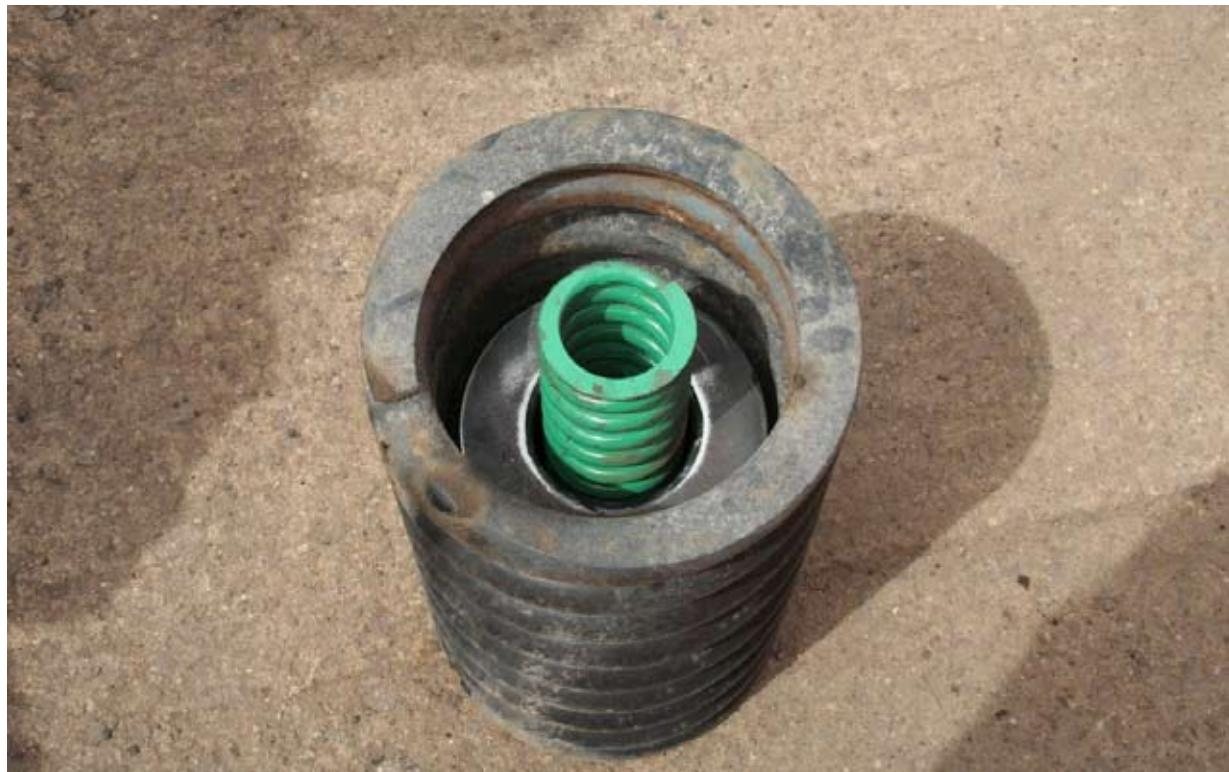
Figure 31: Spring assembly showing primary, secondary and inner 'cup' spring sitting within the 'top hat' component. Inner cup spring is identical that found at Hawks user worked crossing
