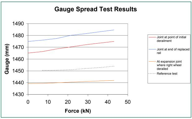
Figure 8: Gauge spread bar tests
