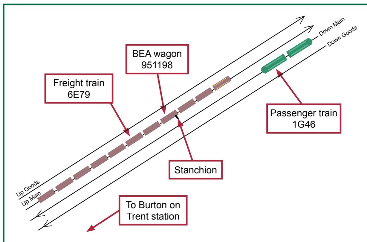
Figure 2: Trains 1G46 & 6E79 before the collision
