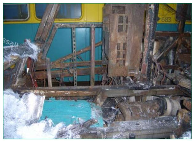
Figure 5: Fire damage to the B end driving position
