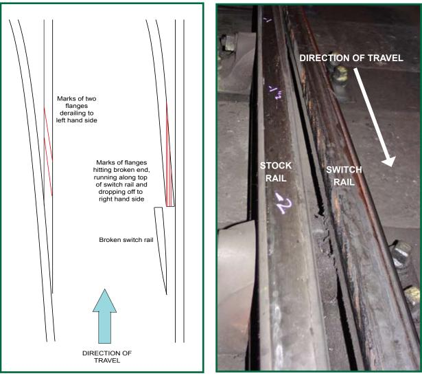
Figure 5: Derailment marks on the rails of points 8A.
