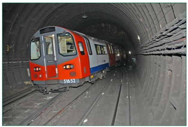
Figure 2: The derailed train seen from the rear.
