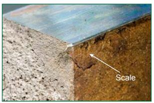
*Figure 8: Detail of fracture origin and adjacent 'scale' at edge.*
