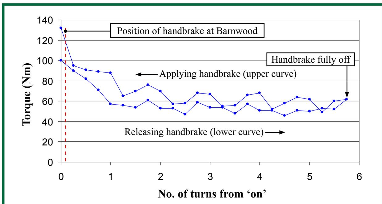
Figure 20: Observed variation of applied torque with turns of the handbrake wheel on SSA wagon 470028
