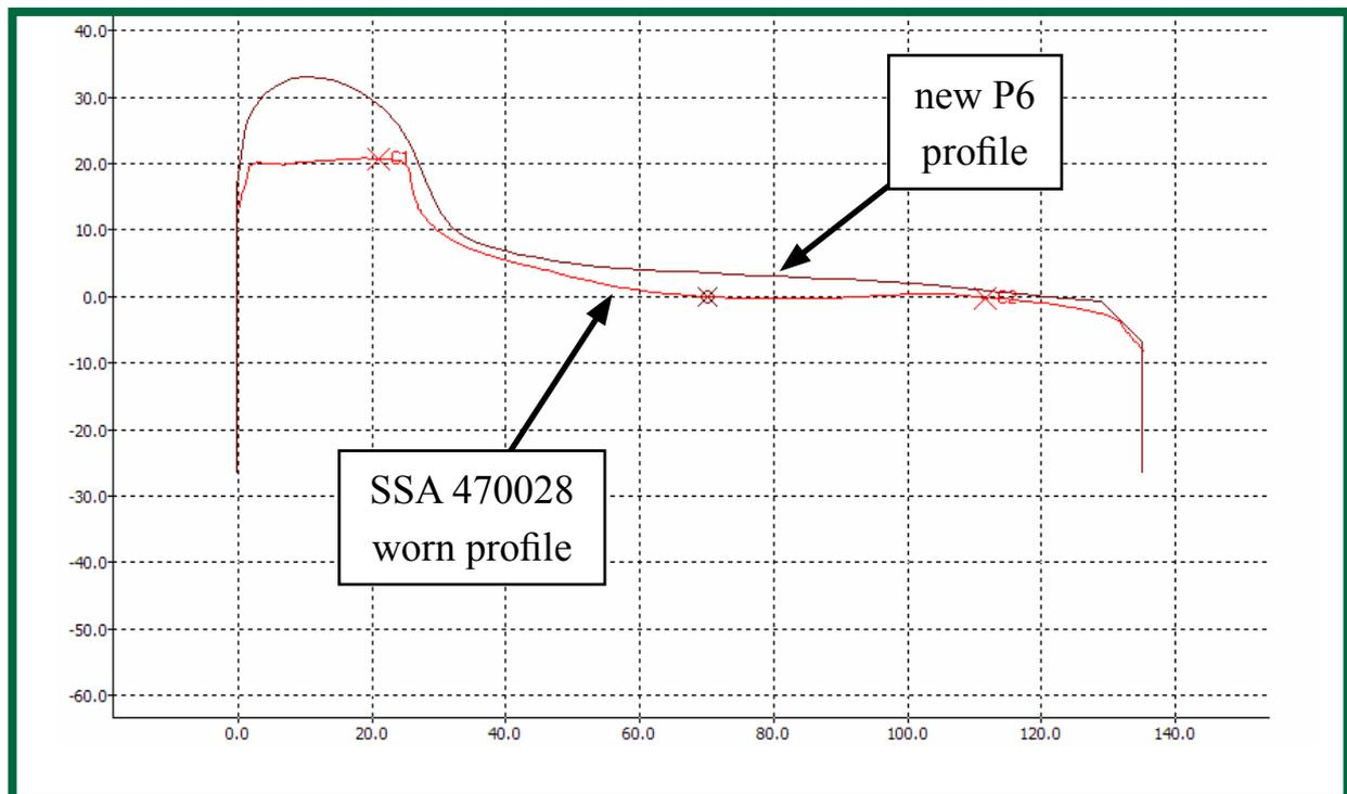
Figure 18: Profile of right leading wheel showing uniform groove pattern due to slow rotation and wear during early part of journey.
