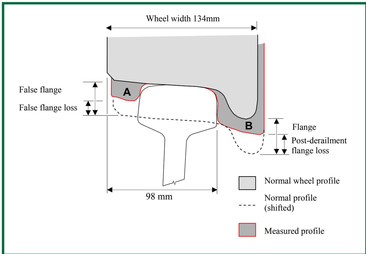
Figure 4: Profile of SSA 470028 Wheel 2A (leading left wheel) and illustration of flattened wheel profile wrapping around the rail head. The false flange is indicated at **A**, and the increased flange depth is shown on the opposite side at **B**.
