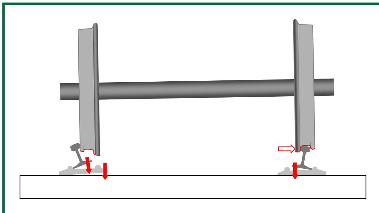
Figure 7: One sleeper after point of derailment. High lateral forces are developed by track's resistance to gauge spreading following partial derailment of left wheel. A 98 mm effective gauge increase was accommodated by lifting of baseplates and failure or displacement of 'Pandrol clips' (see Appendix B), resulting in outwards rotation of left rail.
