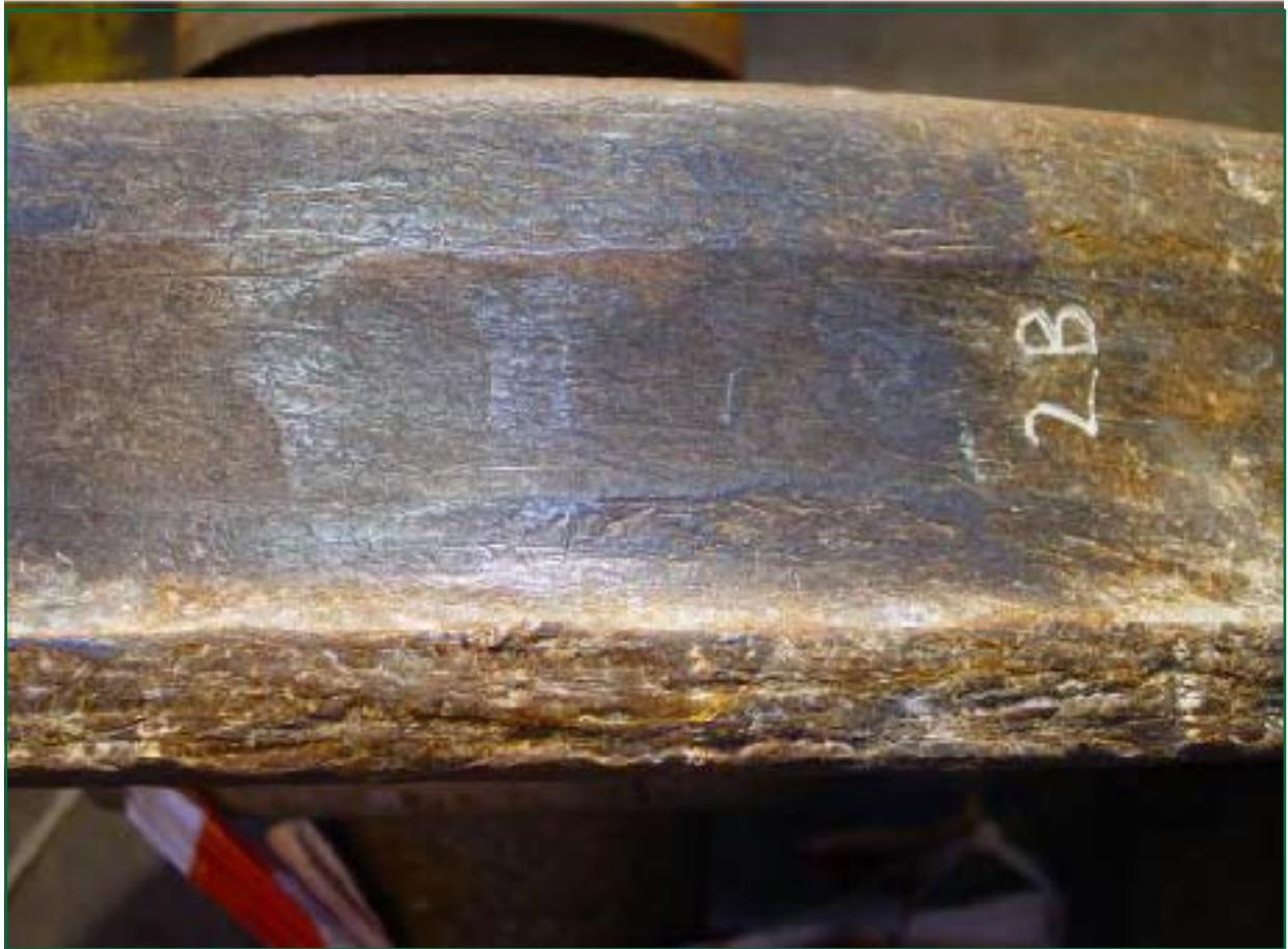
*Figure 19: Surface the uniform groove, visible after gentle burnishing.*
