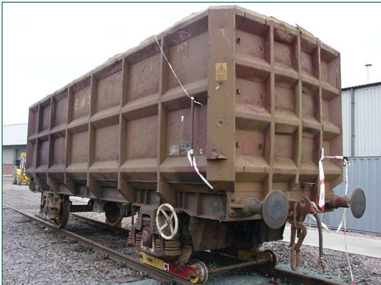
Figure 12: SSA 470028 after recovery to Toton Depot with wheel skate (marked C1) used to move the wagon with its damaged wheelset after the derailment
