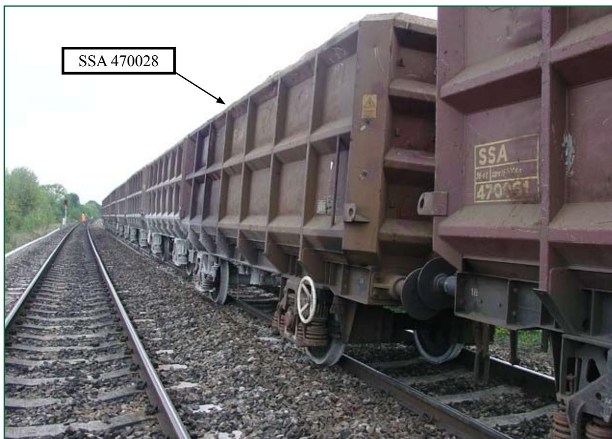
Figure 2: SSA 470028 after derailment
