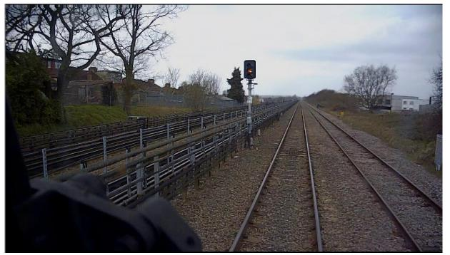
Figure 5: signal GE57 showing yellow (caution). The signal was incorrectly plated G57 at the time of the incident, but this has since been corrected.
