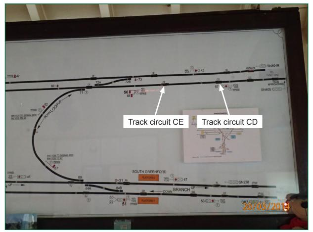
Figure 9: Signal box diagram at Greenford (part), showing down main line approach
