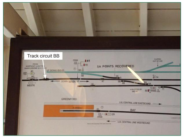
Figure 14: Part of Greenford signal box diagram, showing the line to Northolt Junction
