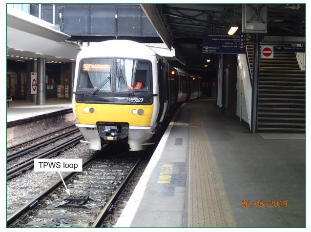
Figure 11: Two-car class 165 drawn up the stop block in platform 14 at Paddington, showing TPWS trigger loop clear of west end cab
