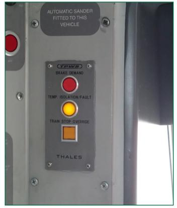
Figure 12: TPWS control panel in unit 165026
