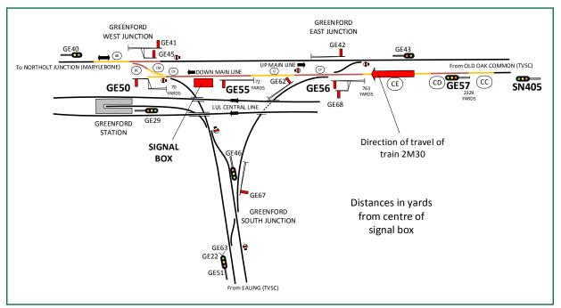
Figure 2: Greenford area, showing track layout and signals
