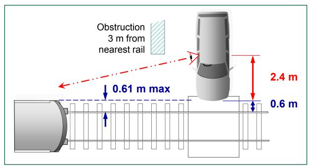
Figure 14: Diagram showing clearance for large car with driver's eye three metres from nearest rail
