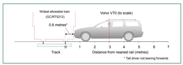
Figure 15: Diagram of large car with driver's eye position 3 metres from nearest rail
