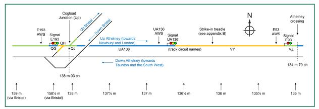
Figure 3: Track layout, showing signals and track circuit names on the Up Athelney line
