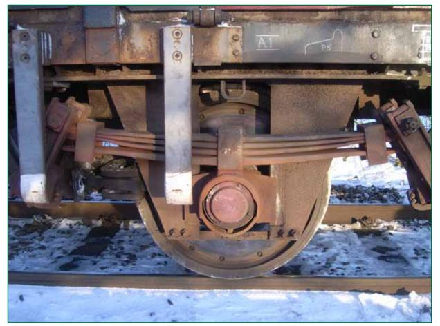
Figure 6: Parabolic leaf spring suspension
