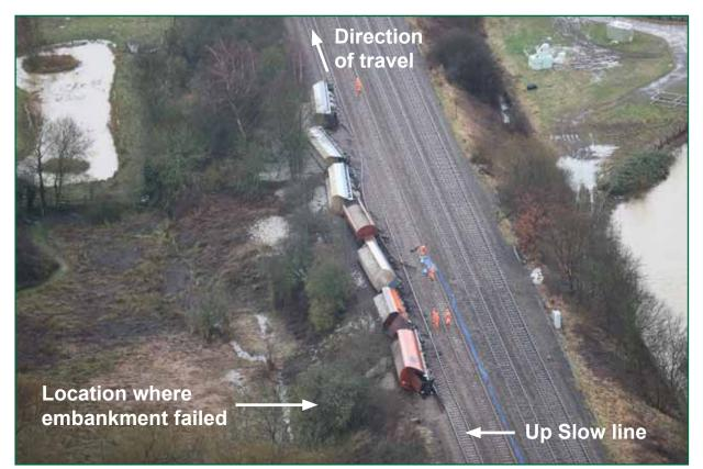
Figure 2: Aerial view of the accident site (photograph courtesy of Network Rail)
