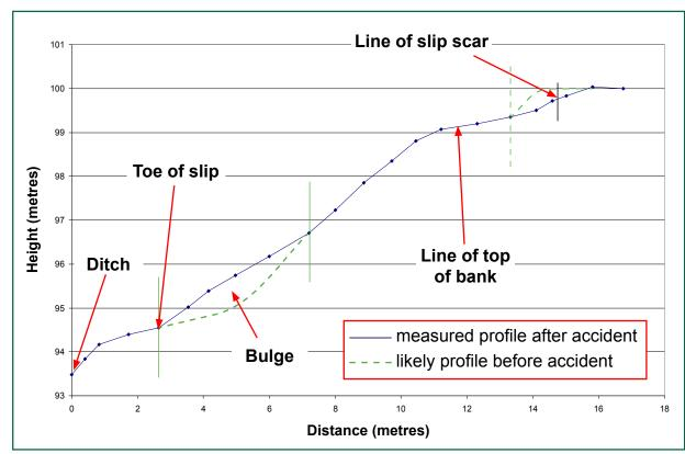
Figure 9: The embankment profile after the failure
