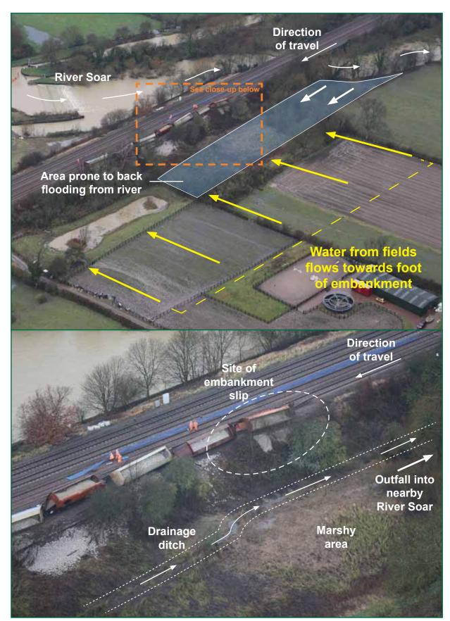
Figure 13: Drainage from the foot of the embankment to the River Soar (photographs courtesy of Network Rail)
