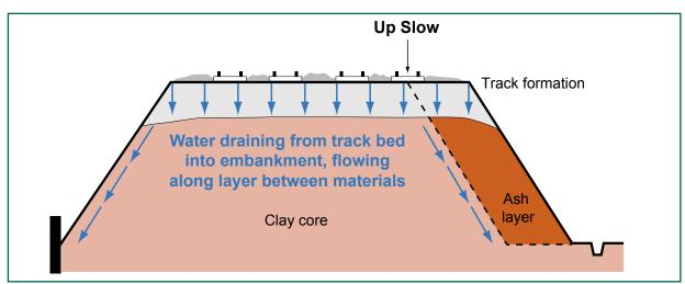
Figure 11: The layers within the embankment
