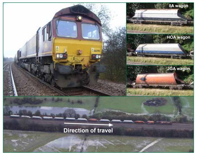
Figure 4: Class 66 locomotive (above left); IIA, HOA and JGA wagons (above right); and Train 6L73 (below - photograph courtesy of Network Rail)
