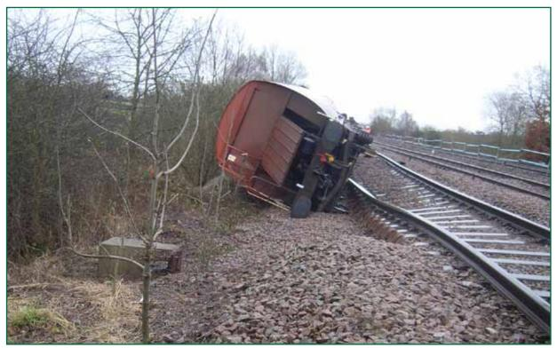
Figure 7: The rearmost wagon and loss of support under the cess rail of the Up Slow line
