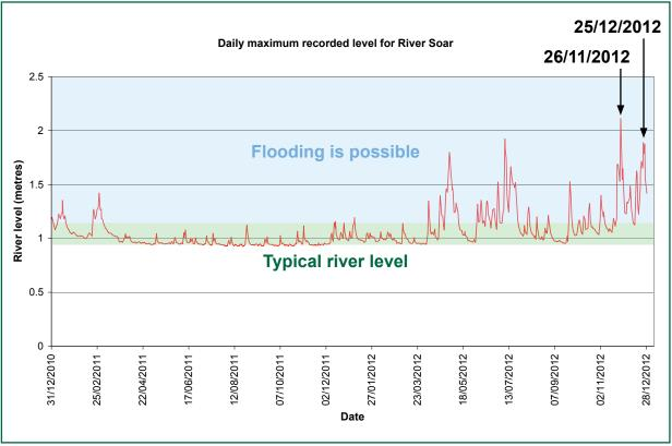
Figure 14: Graph showing level of River Soar recorded at Pilling's Lock for 2011 and 2012
