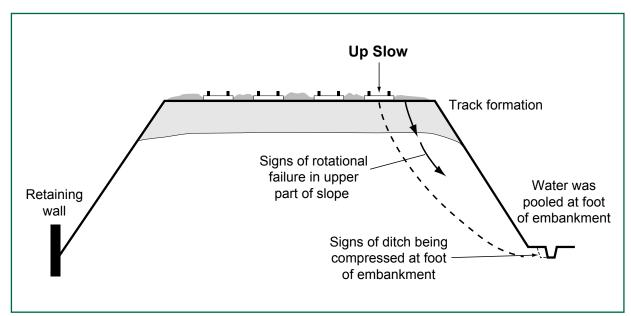
Figure 10: The rotational failure within the embankment
