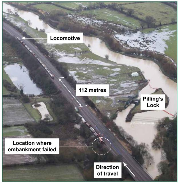
Figure 6: Where the two portions of train 6L73 came to rest (photograph courtesy of Network Rail)
