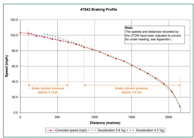
Figure 7: 47843 braking profile
