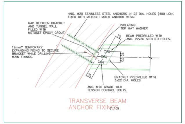
Figure 6: Scott Wilson's design drawing showing transverse beam end fixing
