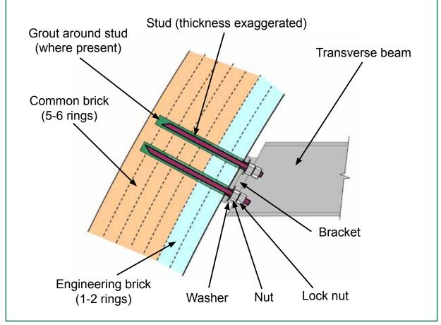
Figure 7: Simplified diagram of transverse beam end fixing
