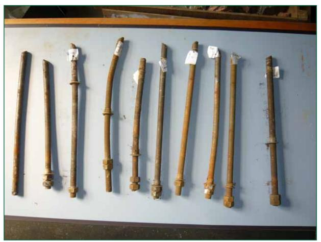
Figure 17: Selection of missing studs found in the tunnel - note variation in length
