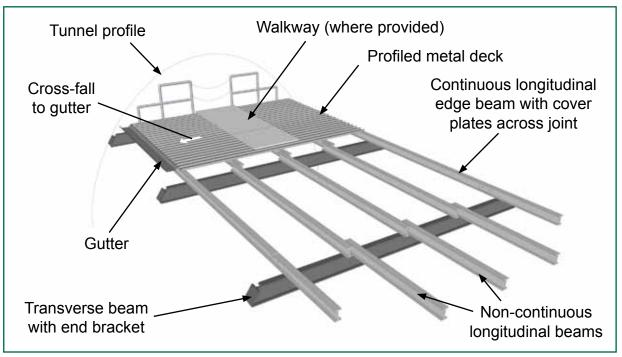
Figure 4: Diagram of water catchment tray structure
