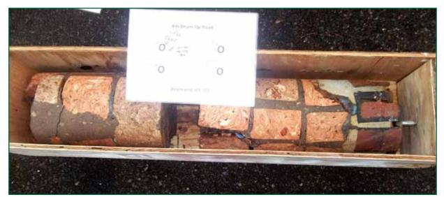
*Figure 15: Core taken from tunnel lining during investigation, showing engineering brickwork (right). Core split into two sections during removal (photograph courtesy of Network Rail).*
