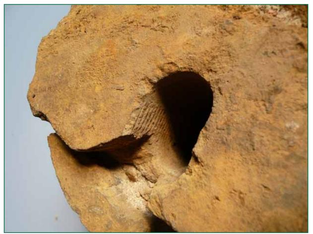
Figure 14: Deformed hole in brickwork core removed from tunnel lining
