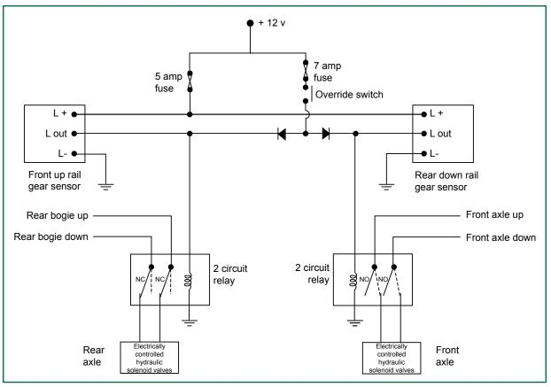
Figure 11: Axle interlocking circuit diagram for dumpers 216 and 217, as designed (information from hand-drawn diagram supplied by Quattro)
