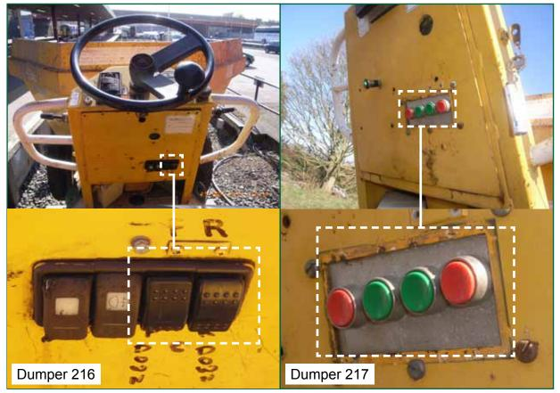
Figure 16: Rail axle control switches on dumpers 216 and 217
