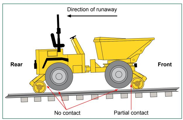
Figure 10: Positions of the road and rail wheels following the accident
