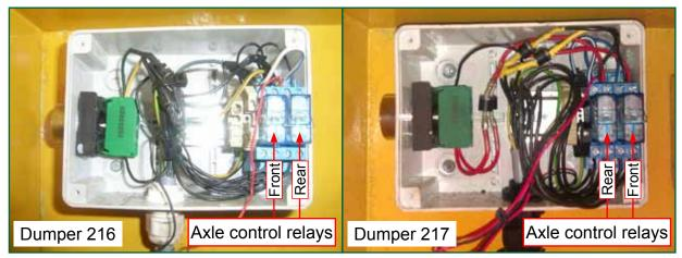
Figure 14: Views inside dumper 216 and 217 interlocking electrical circuit boxes
