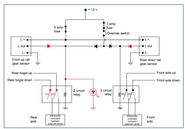
Figure 13: Actual axle interlocking circuit diagram for dumper 217
