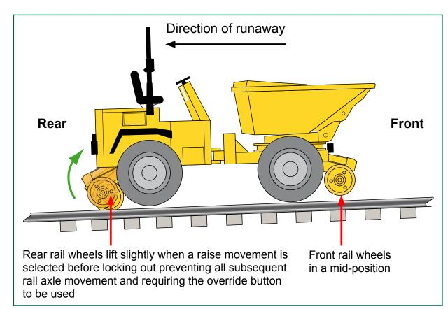
*Figure 8: Effect of selecting an out-of-sequence movement of the rail axles when off-tracking dumper 216*
