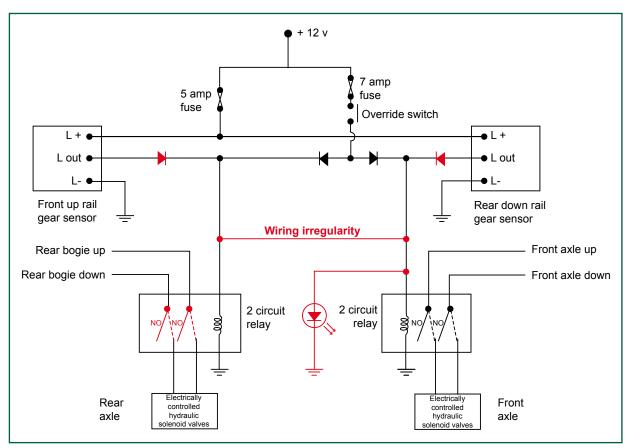
Figure 12: Actual axle interlocking circuit diagram for dumper 216
