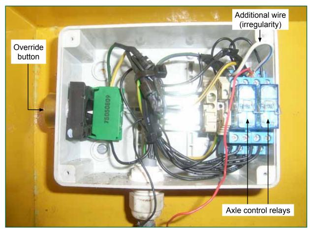
Figure 9: A view inside the axle interlocking circuit box on dumper 216
