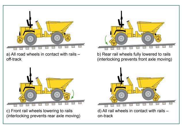
Figure 5: Rail axle movement sequence when on-tracking
