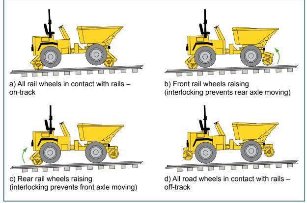
Figure 6: Rail axle movement sequence when off-tracking
