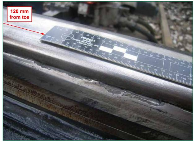
Figure 7: Left-hand switch rail damage
