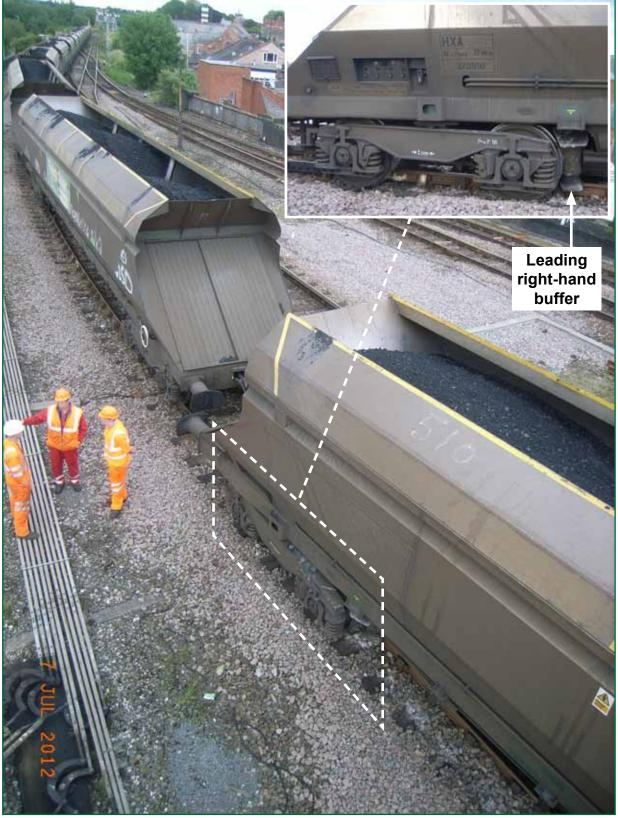
Figure 2: Wagon 370510 after the derailment
