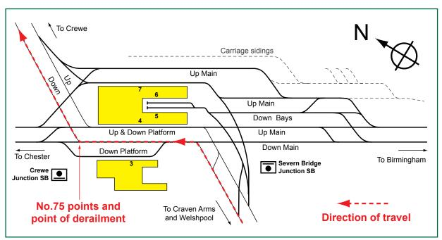
Figure 3: Schematic diagram showing location of accident
