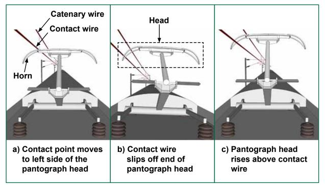
Figure 3: Illustration of process of dewirement
