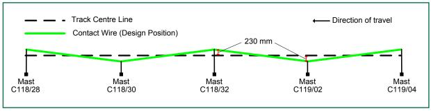
Figure 10: Overhead line designed stagger at accident location
