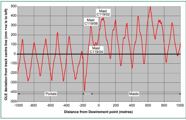
Figure 25: Overhead alignment recorded by MENTOR coach
