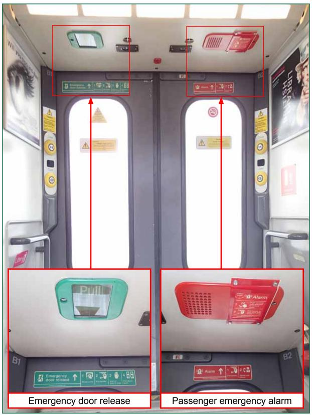
Figure A1: PEA and emergency door release handles
