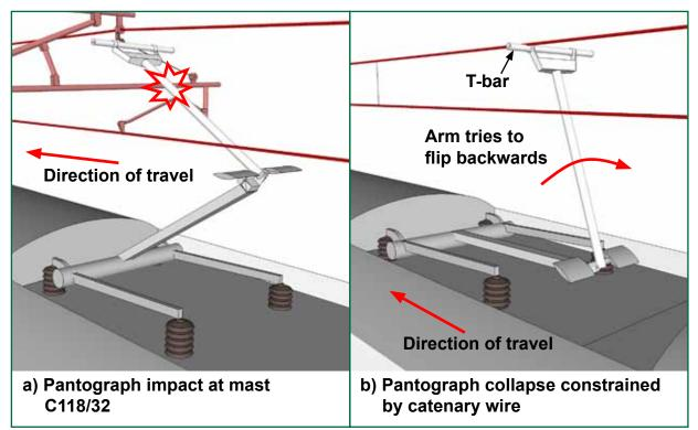
Figure 15: Illustration of pantograph failure sequence (continued)
