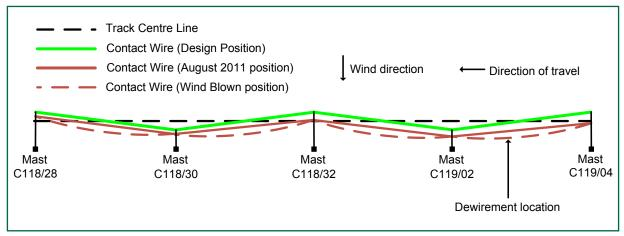
Figure 16: Overhead line alignment at accident location (plan view not to scale)
