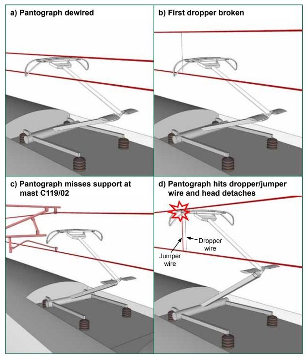
Figure 14: Illustration of pantograph failure sequence
