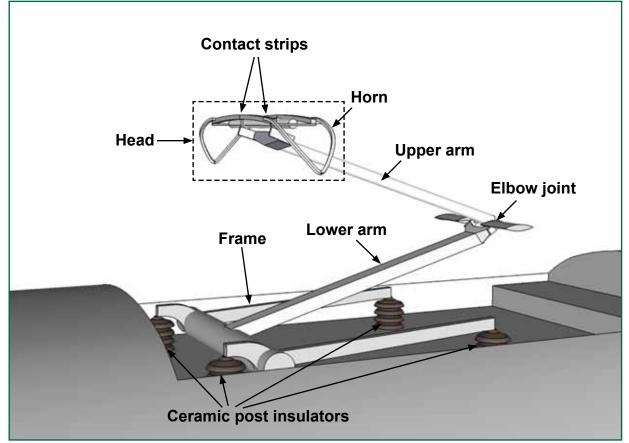
Figure 8: Illustration of train pantograph
