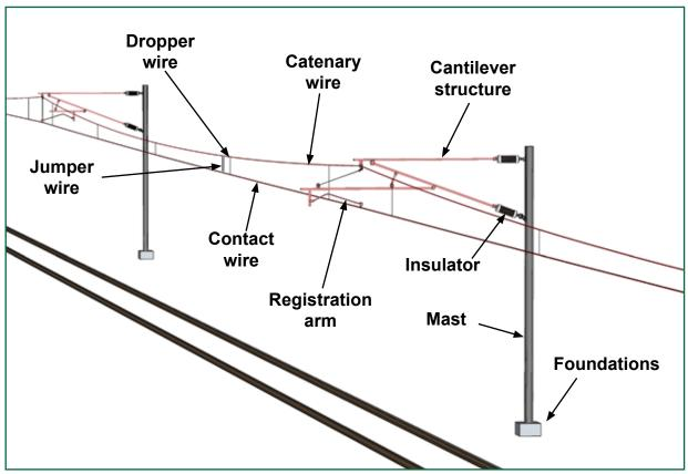
Figure 9: Illustration of overhead line detail
