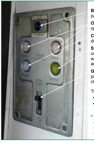
Blue door interlock light: this is lit when all passenger doors are fully closed
