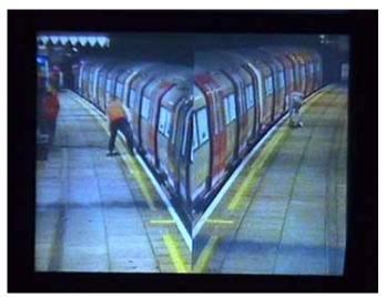
Figure 15: In-vehicle monitor
