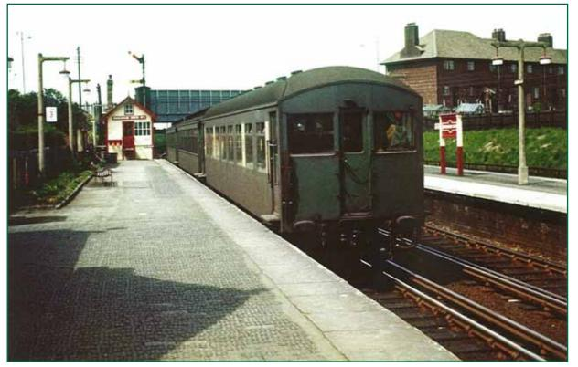
*Figure 24: 1906 stock at Birkenhead North station in 1955 (Copyright Ray DeGroote/Online Transport Archive)*
