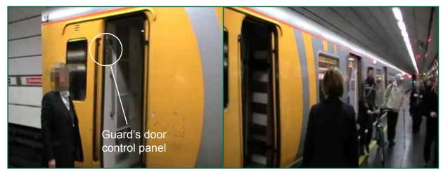
Figure 7: A guard carrying out a safety check
