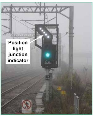
Figure 6: Signal fitted with a position light junction indicator (showing the junction ahead of the signal is set for a diverging movement to the left)
