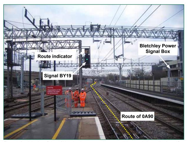
Figure 2: Daylight view of signal BY19 showing a proceed aspect and the route indicator illuminated for a move from the up slow line to the up fast line
