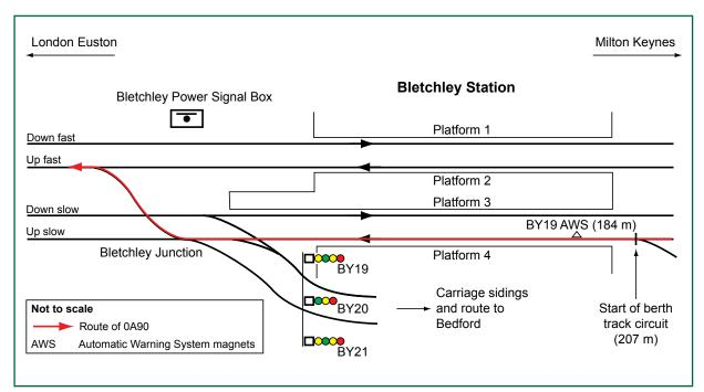
Figure 4: Track layout of Bletchley Junction (distances shown are from BY19 signal)
