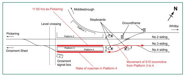
Figure 3: The track layout at Grosmont station
