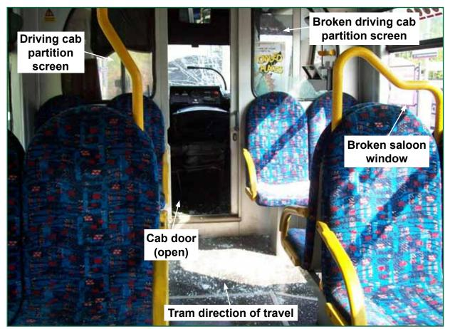
Figure 4: Damage to the saloon interior at the leading end of Tram 13 - the cab door is shown in the open position (image courtesy of National Express Midland Metro)
