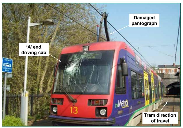
Figure 3: Damage to the trailing end of tram 13 (image courtesy of National Express Midland Metro)
