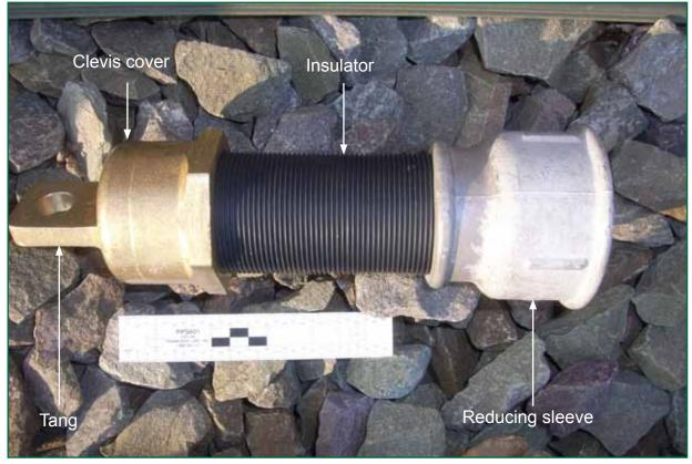
Figure 6: Bracket foot assembly
