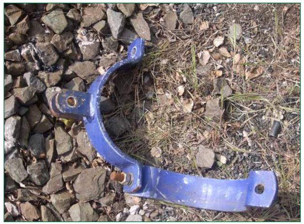
Figure 19: An example of a modified design of pole bracket
