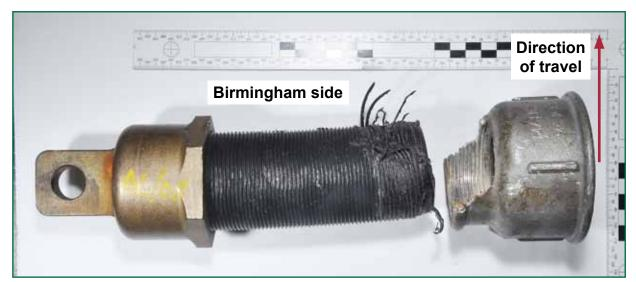
Figure 14: Damage to the bracket foot assembly of 18512 pole
