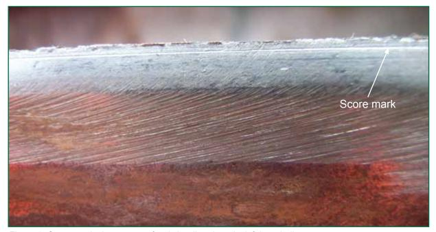
Figure 9: Score mark close to top of switch rail and marks left by grinding
