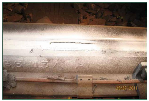
Figure 7: Crack in left-hand switch rail of points 167B at 1.5 metres from switch toe
