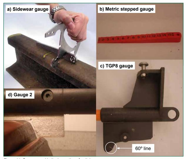
Figure 14: Gauges used in the inspection of switches
