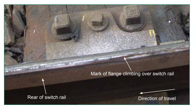
Figure 8: Witness mark of wheel flange climbing over switch rail at 2.8 metres from switch toe
