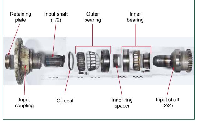
Figure 9: Components of the drive shaft input assembly following failure of the shaft
