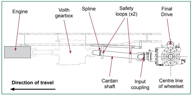
Figure 3: Drive arrangement on Class 14x
