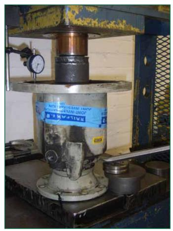
Figure 11: End float measuring technique
