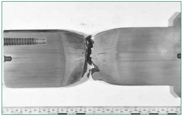
Figure 8: Section through the input shaft
