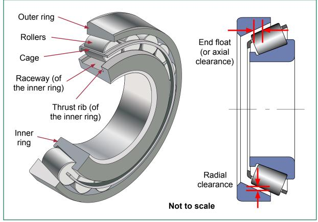
Figure 5: Tapered roller bearing
