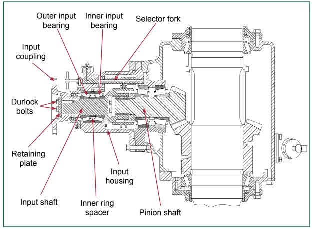
Figure 4: Final drive cross-section
