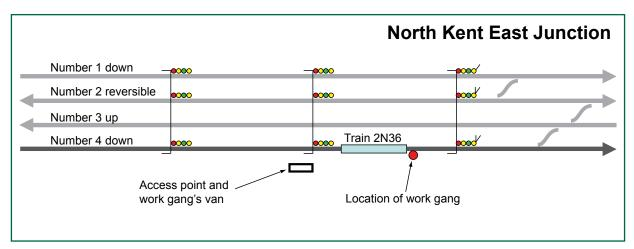
Figure 1: Simplified layout of the approach to North Kent East Junction showing the location of the work gang, and the approach of train 2N36 (not to scale).
