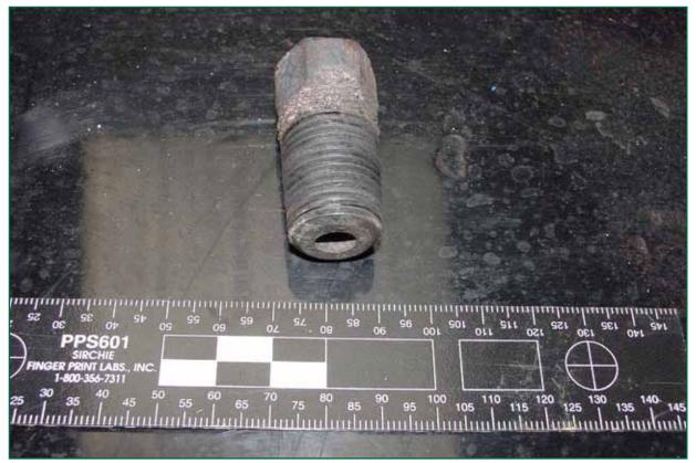
Figure 6: Fusible plug removed from 'Hawk'
