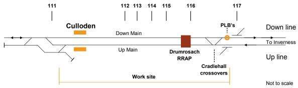
Figure 6: Track plan showing the possession and worksite limits for 20 July 2010
