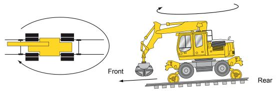
**Figure 14 r - s** - The machine operator quickly swings the cab to the front of the RRV (in the direction of travel).
