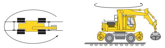
Figure 9 c & d - The cab is swung to the rear of the RRV and the rear rail wheels are lined up with the track using the road wheels to manoeuvre the machine.
