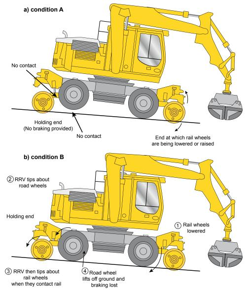
Figures 8a and 8b: High-ride RRV - on/off-tracking runaway conditions
