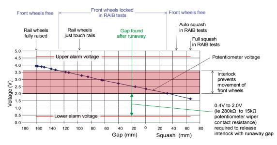
Figure 11: Graph showing relationship between voltage and road/rail wheel air gap
