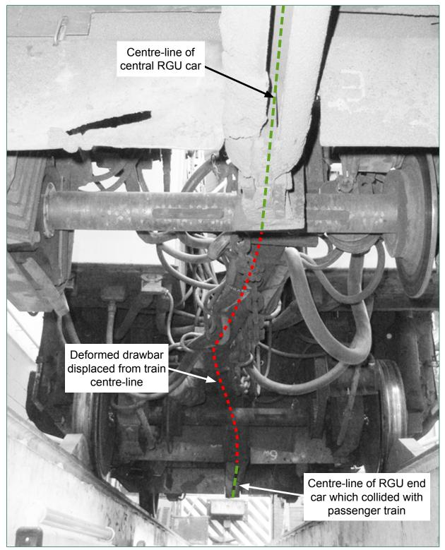
Figure 18: Deformed drawbar on RGU.
