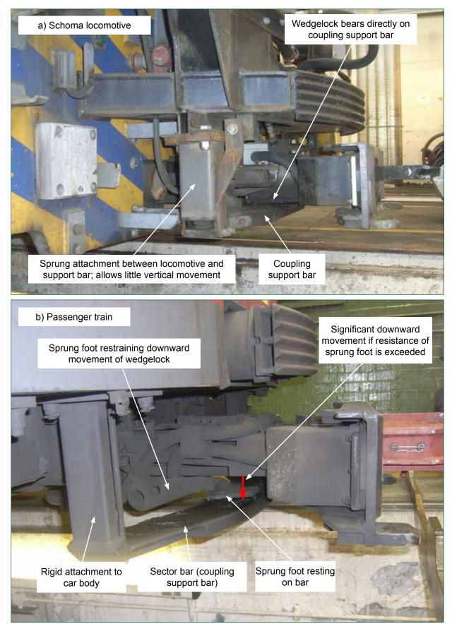
Figure 20: Wedgelock vertical rotation.
