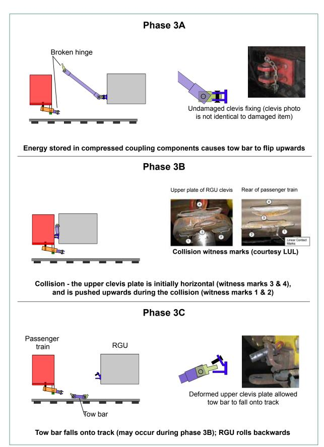
Figure 17: Upward tow bar movement (phase 3 of breakage).
