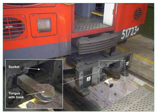
Figure 10: Wedgelock coupler.
