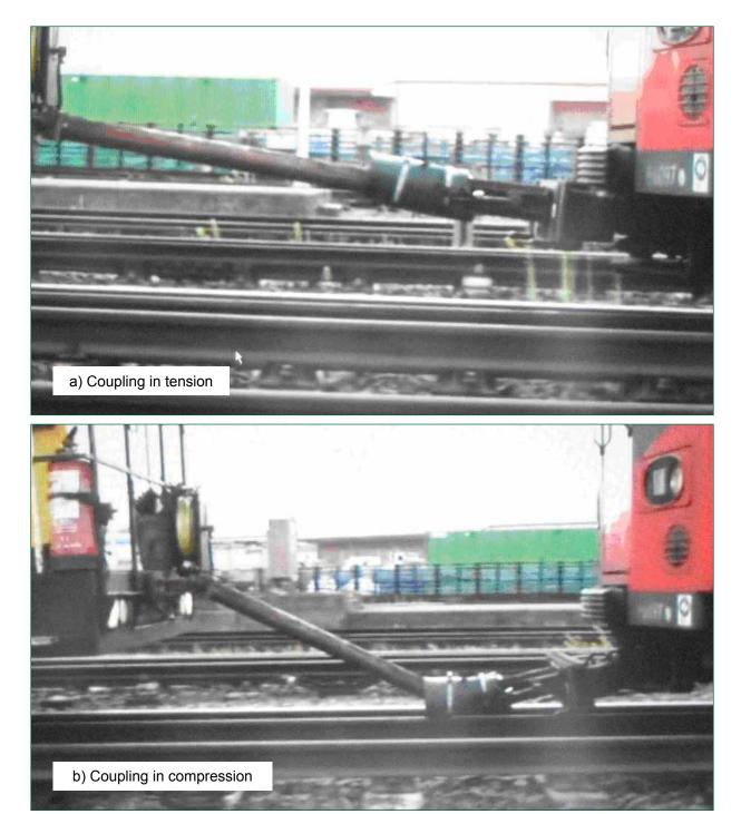
*Figure 14: Vertical coupling deflection observed during July 2010 testing (images from video provided by Tube Lines).*
