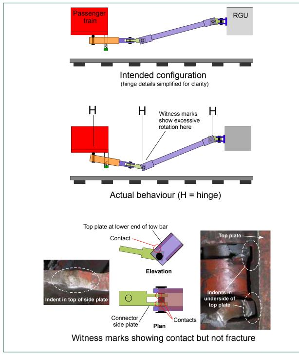
Figure 13: Vertical coupling deflection (phase 1 of breakage).
