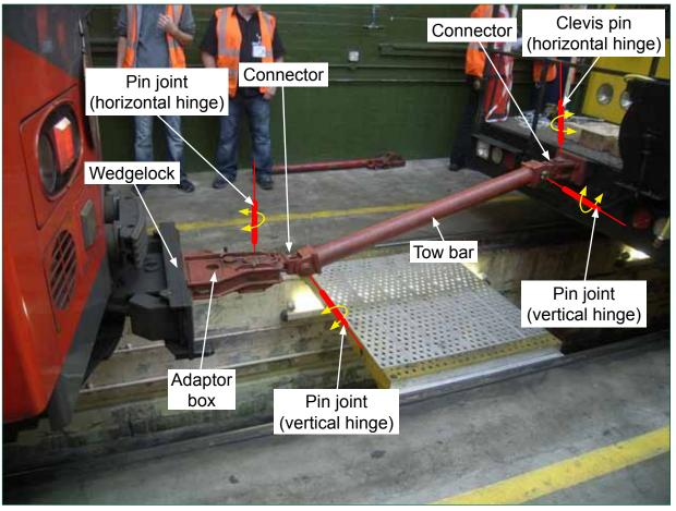
Figure 12: Emergency coupler components.
