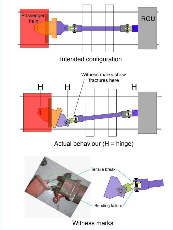
Figure 15: Lateral coupling deflection (phase 2 of breakage).
