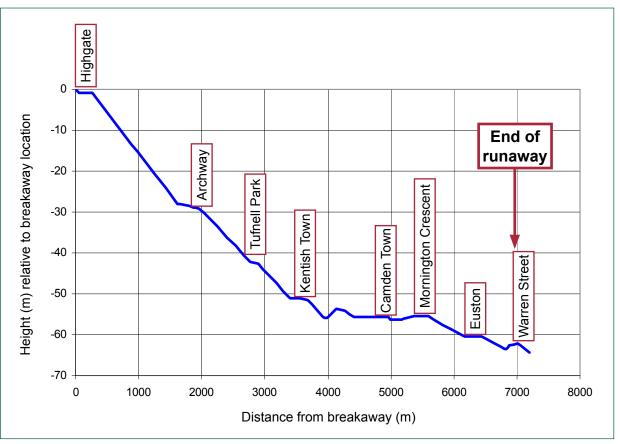
Figure 2: Northern Line vertical alignment.
