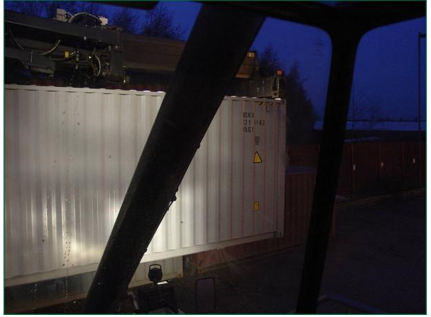
Figure 10: View from cab of reach stacker showing restricted vision after dark and black/yellow stripes on top corner of high-cube container
