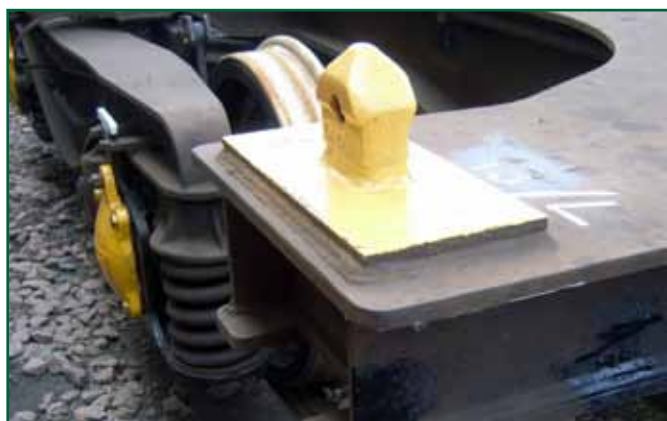
Figure 12: Example of fixed UIC spigot (FEA-A wagon)
