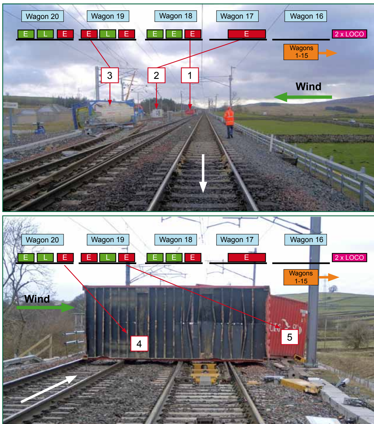
Figure 4: Detached containers at Hardendale and their original location on train 4S83 (white arrows denote direction of travel)
