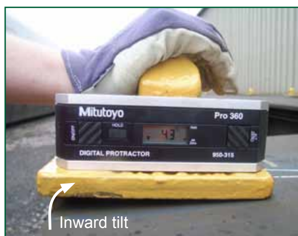
Figure 14: Inward rotation of fold-down UIC spigot with outboard hinge, due to play in hinge
