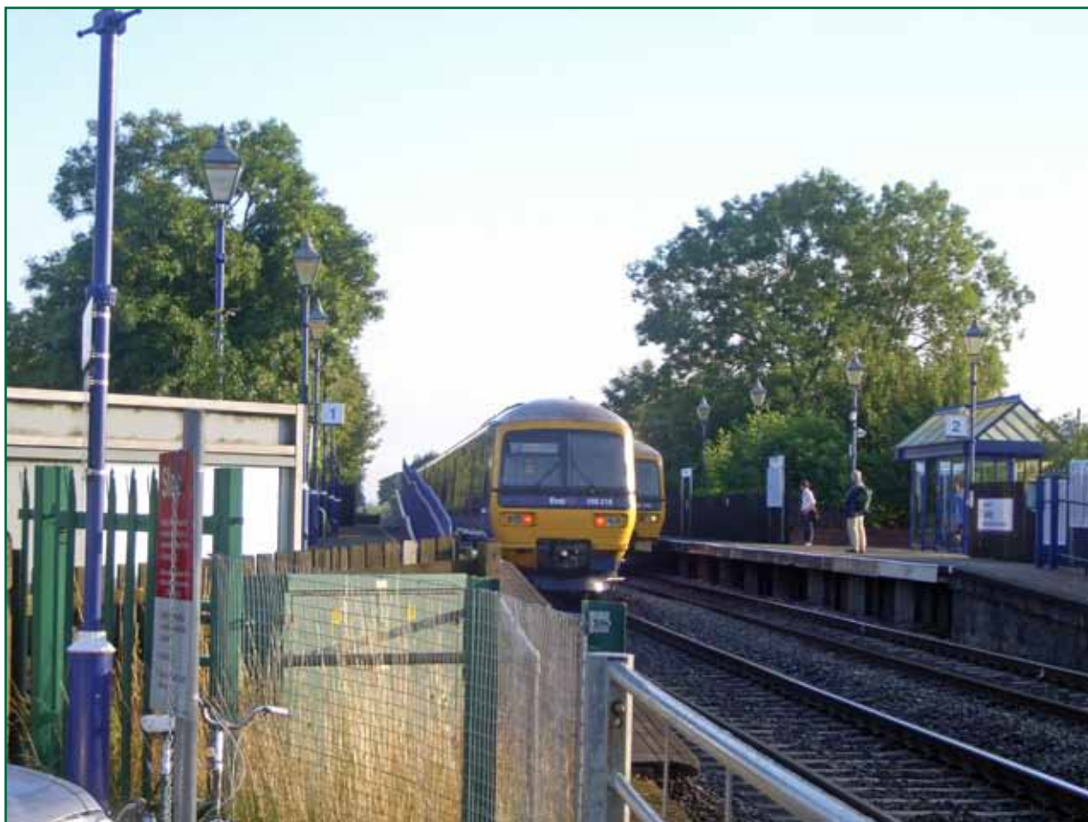
Figure 11: Photograph of train in down platform, in August 2008, illustrating the 'hidden train factor'. Note that the green palisade fence has now been removed, but that sighting is still affected by fencing on the platform
