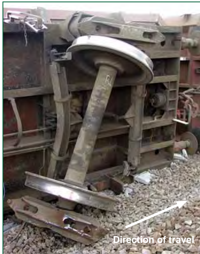
Figure 8: Damage to the left leading suspension of wagon 470152
