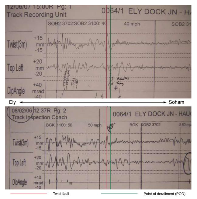
Figure 27: Track recording vehicle data trace from 8 February 2006 (bottom) and 12 June 2007 (top). The horizontal dotted line indicates the intervention limit. The track twist and POD are also shown Report 02/2009 36
