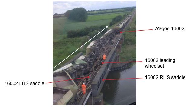
Figure 12: View of derailed wagons on bridge 2235
