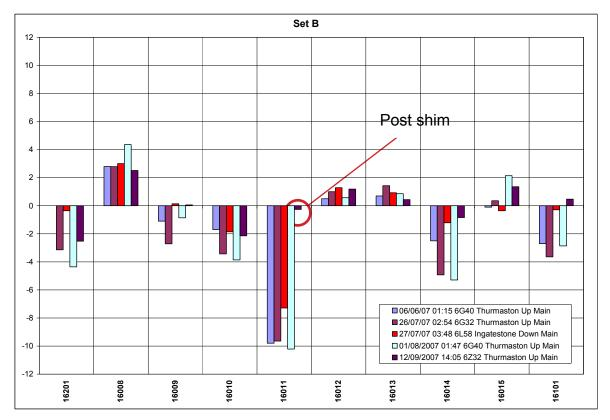
Figure 39: Graph showing analysis of raw Wheelchex data of pre and post frame twist on REDA 16011
