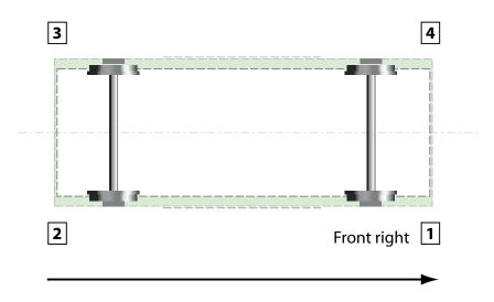
Figure 6: Plan view of PHA wagon with front right and left axle 1 - 4 and rear axle 2 - 3
