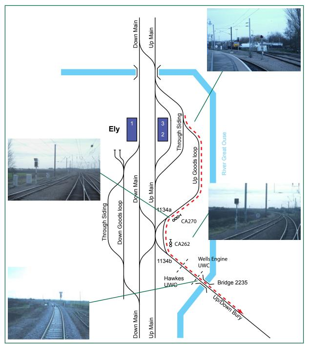
Figure 2. Plan showing signals passed by the train in the Ely area, and incorporating images of the route
