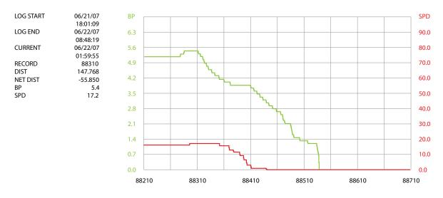
*Figure 30: Locomotive 60068 OTDR reading of speed (red trace) and brakepipe pressure (green trace) at 01:59:55 seconds 22 June 2007*
