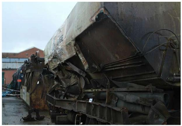
Figure 34: Left side of wagon REDA 16002 showing severe damage and frame twist caused by incident
