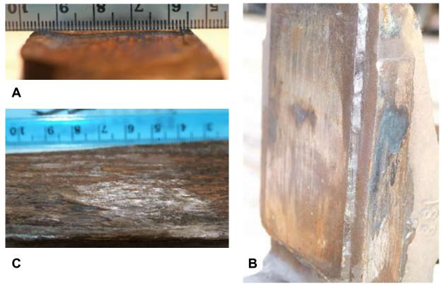
*Figure 49: (A) Image of furrowing from front pedestal of REDA 16002. (B) Image of front portion of inner aspect of leading right-hand pedestal. (c) Heat damage and corrosion to pedestal guide*
