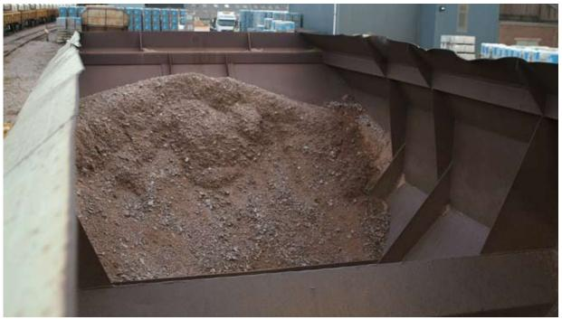
Figure 19: Residual ballast in wagon REDA 16021
