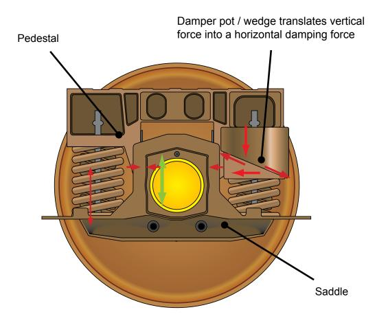
Figures 7: GFA suspension showing damping forces of pedestal and saddle
