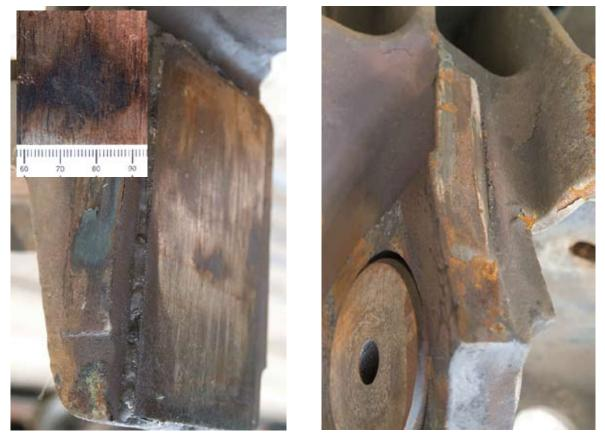
*Figures 32 (left) with inset. Front portion of inner aspect of the right-hand pedestal showing heat damage. Figure 33 (right). Heat damage to rear portion of inner aspect of pedestal guide.*
