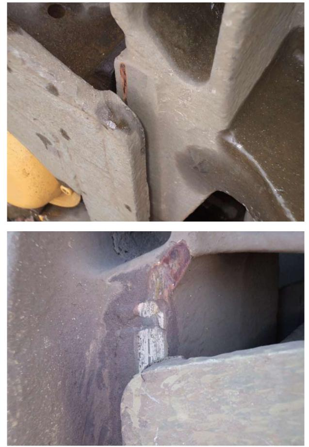
Figures 51 & 52: Wear and heat damage to pedestal liners of SDT PHA wagons
