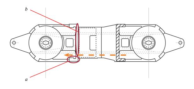
*Figure 50: Plan view of Leading RHS pedestal and saddle showing area of frictional heat generation at (a) lateral guide and (b) friction liner*
