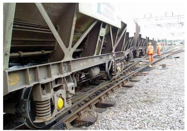
Figure 46: Image showing derailed wagons REDA 16001,16002 and 16003
