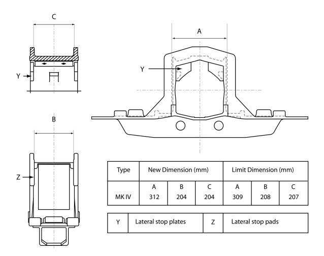
Figure 53: Saddle casting and tolerances
