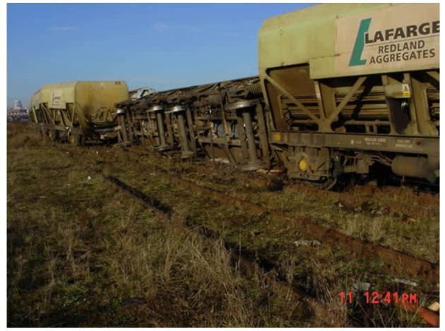
Figure 45: Image showing train 6D38 derailed within Small Heath sidings
