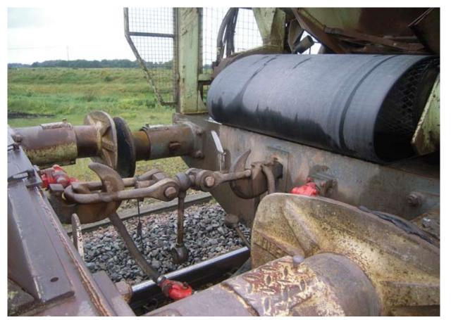
Figure 4: REDA coupling arrangement
