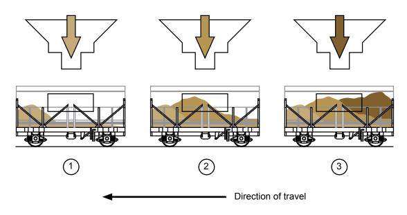
Figure 18: Diagram showing loading procedure and propensity to load wagons rear-axle-heavy
