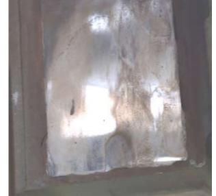
Fig 38: Wear to leading right pedestal guide on REDA 16011 showing polished surfaces but no evidence of heat damage
