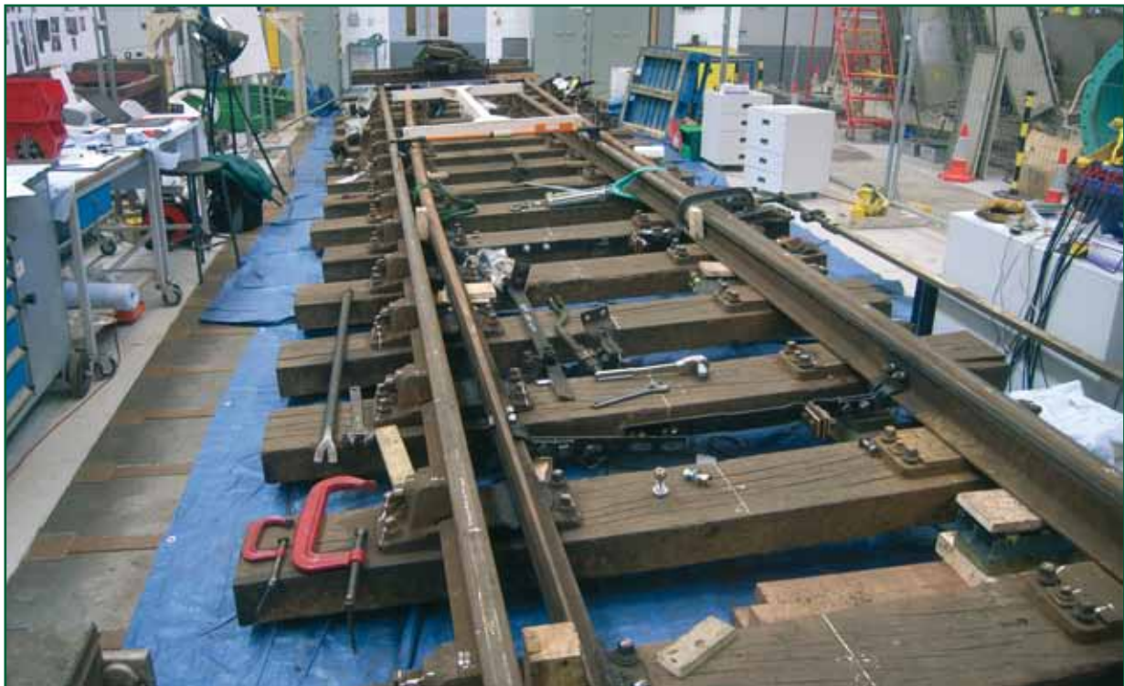
Figure 6: Points 2B switch section in laboratory
