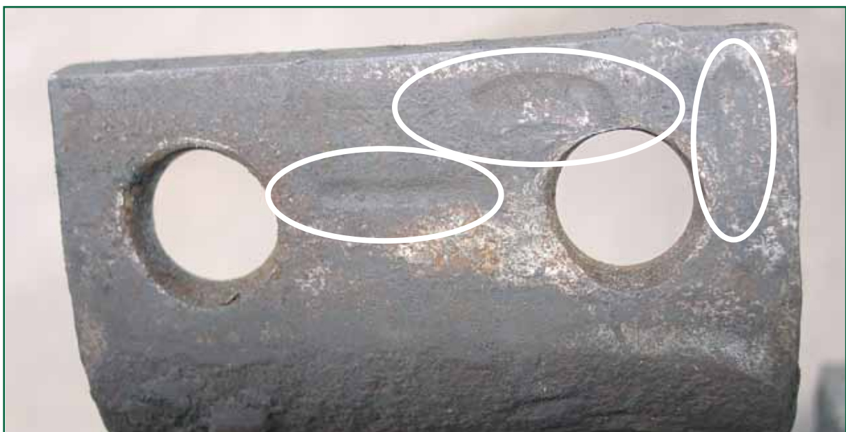
Figure 25: Indentations imprinted into the mating face
