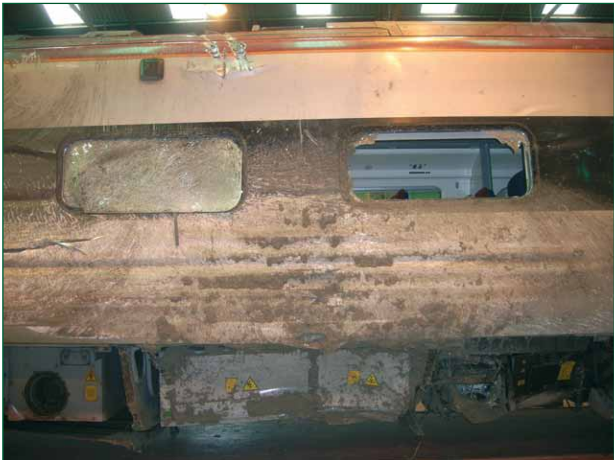
Figure 38: Damaged central section of the left-hand bodyside of vehicle two
