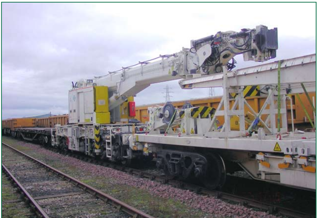
Figure 4: Kirow crane DKR81623 and its match wagon
