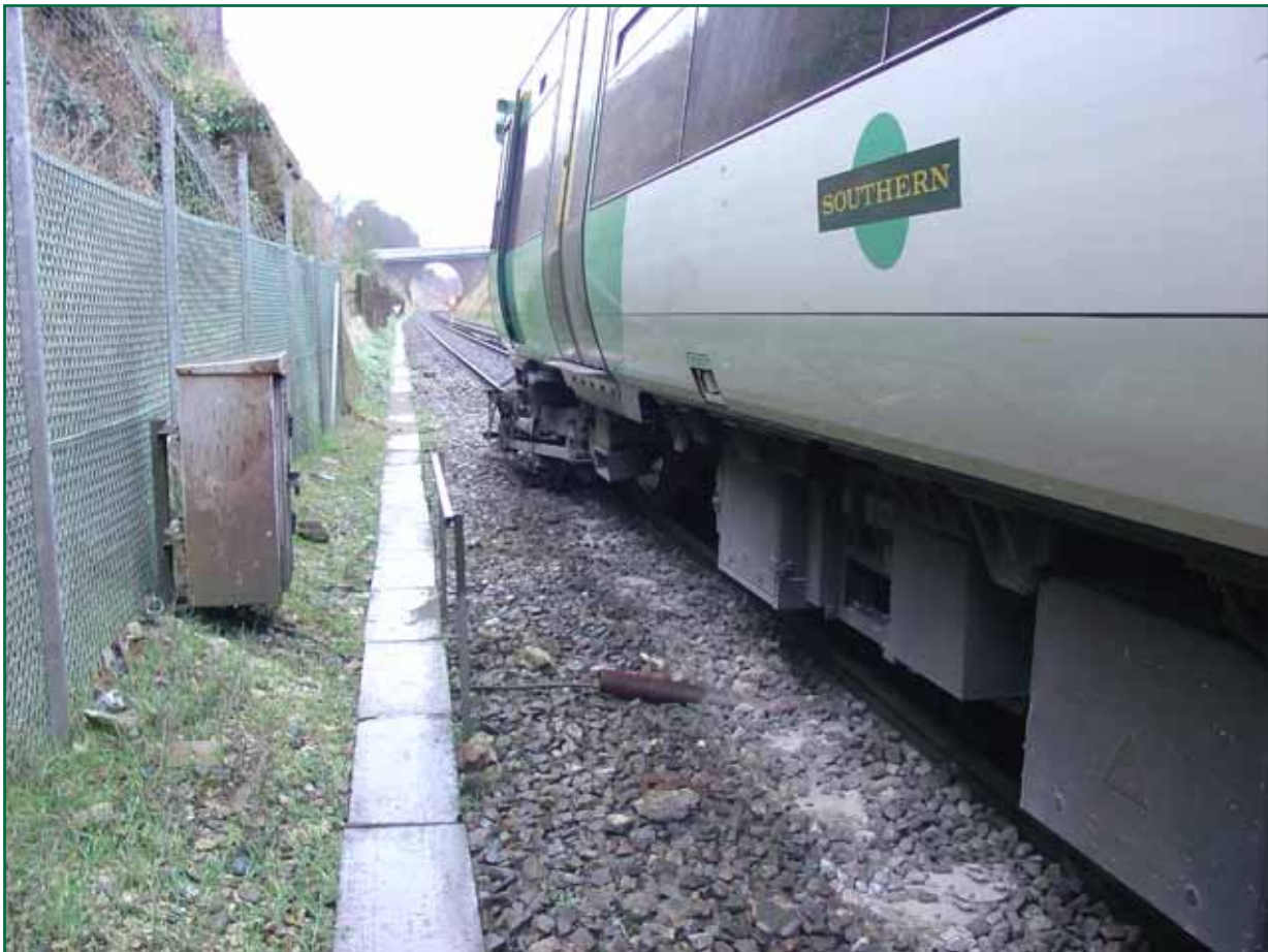
Figure 14: The derailed bogie and side of the train
