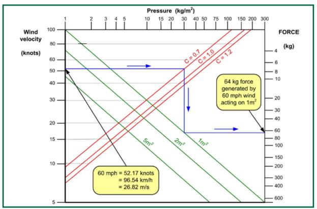
Figure 13: Wind speed and force diagram [Reference 5]
