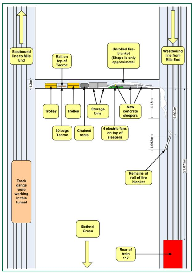
Figure 12: Diagram of cross passage and running tunnels
