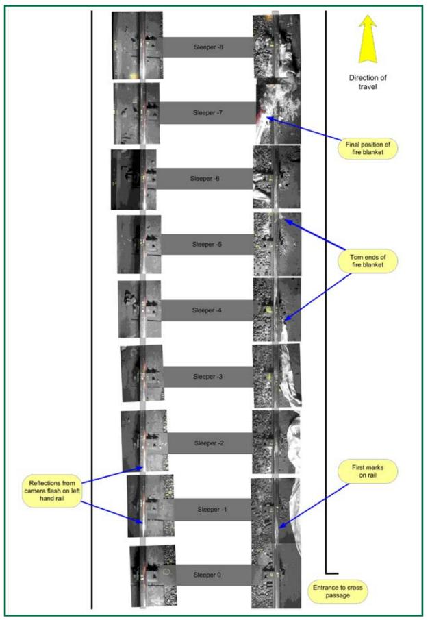
Figure 14: Composite photo diagram showing the rails between the initial point of impact and the final position of the roll of fire-resistant blanket
