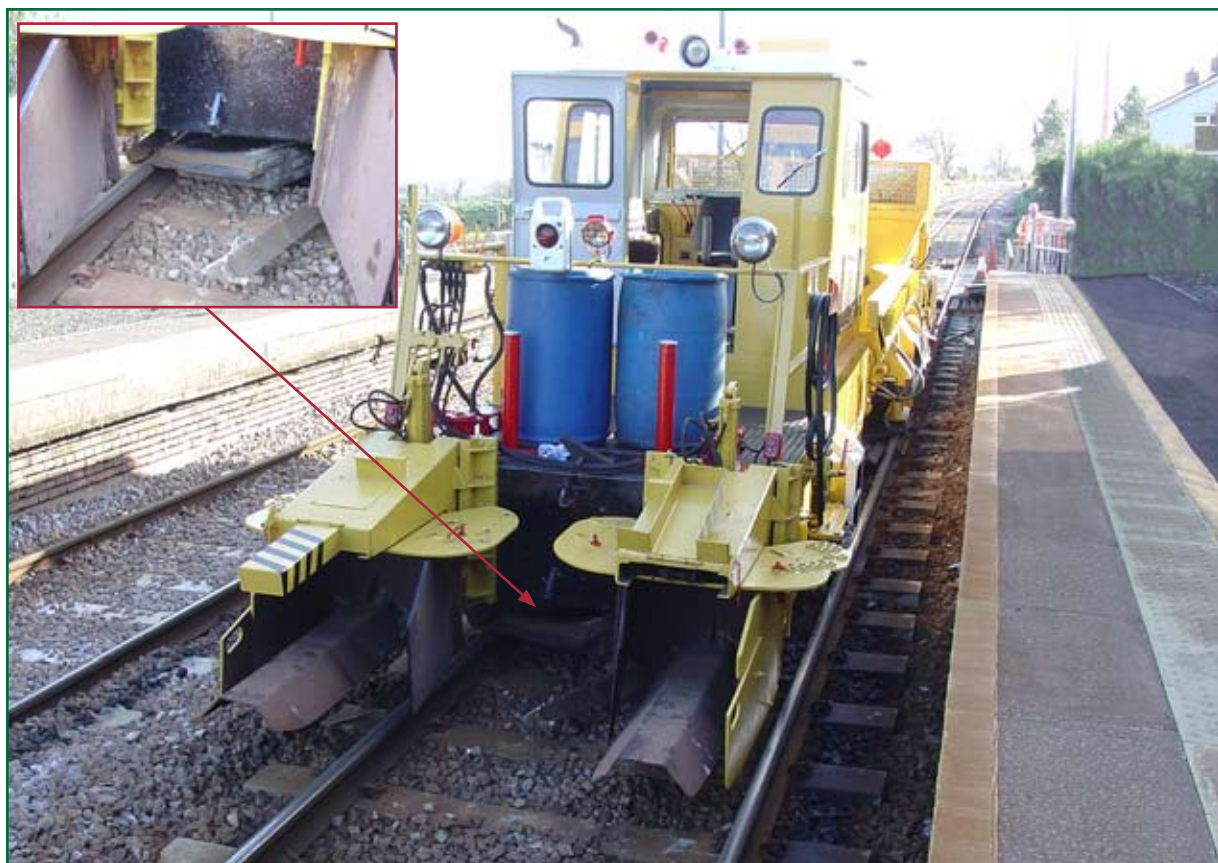
Figure 5: Ballast regulator 315 at Trooperslane station following derailment. The headstock on which both the towing brackets and anchor bracket are mounted is painted black (insert). A displaced road crossing block originating from the level crossing is shown in the background wedged beneath the vehicle
