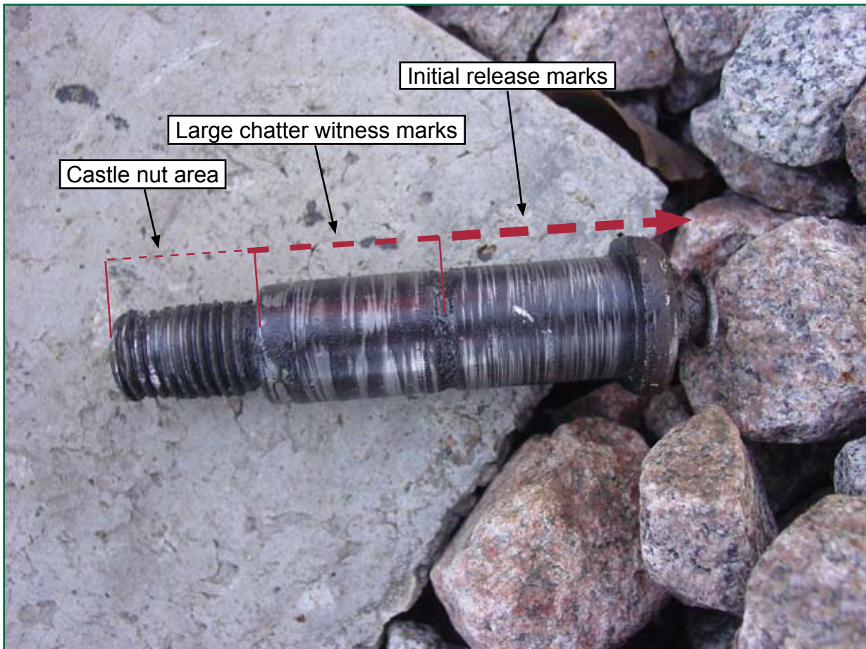
Figure 10: Image of securing pin found on site
