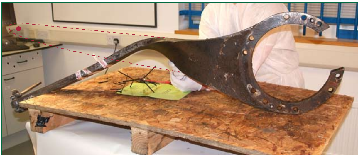
Figure 14: Damaged lower torque arm
