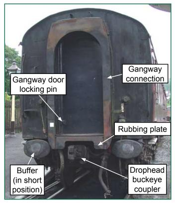
Figure 10: The carriage end showing the external features
