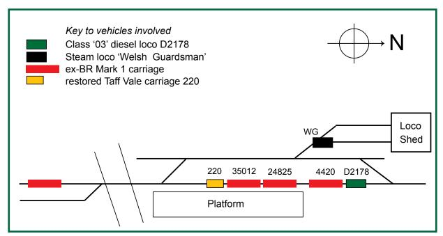
Figure 6: Location of relevant rail vehicles during the during the shunting manoeuvre, immediately prior to the accident occurring
