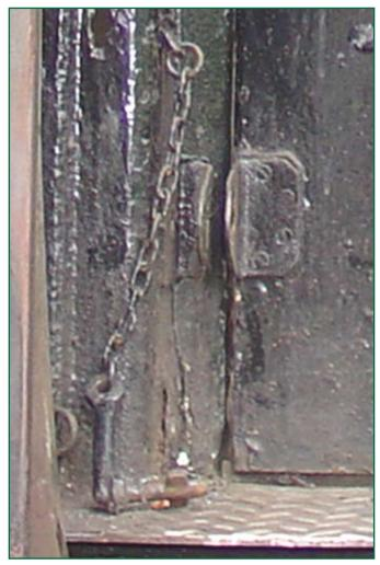
Figure 11: the carriage end door locking pin in the unlocked position
