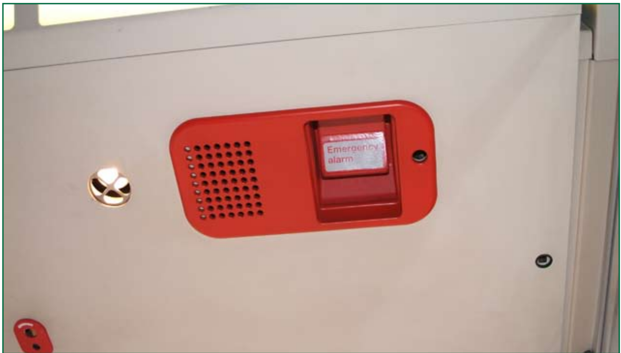
Figure 30: Labelling on the emergency alarm – Class 365 Unit door.
