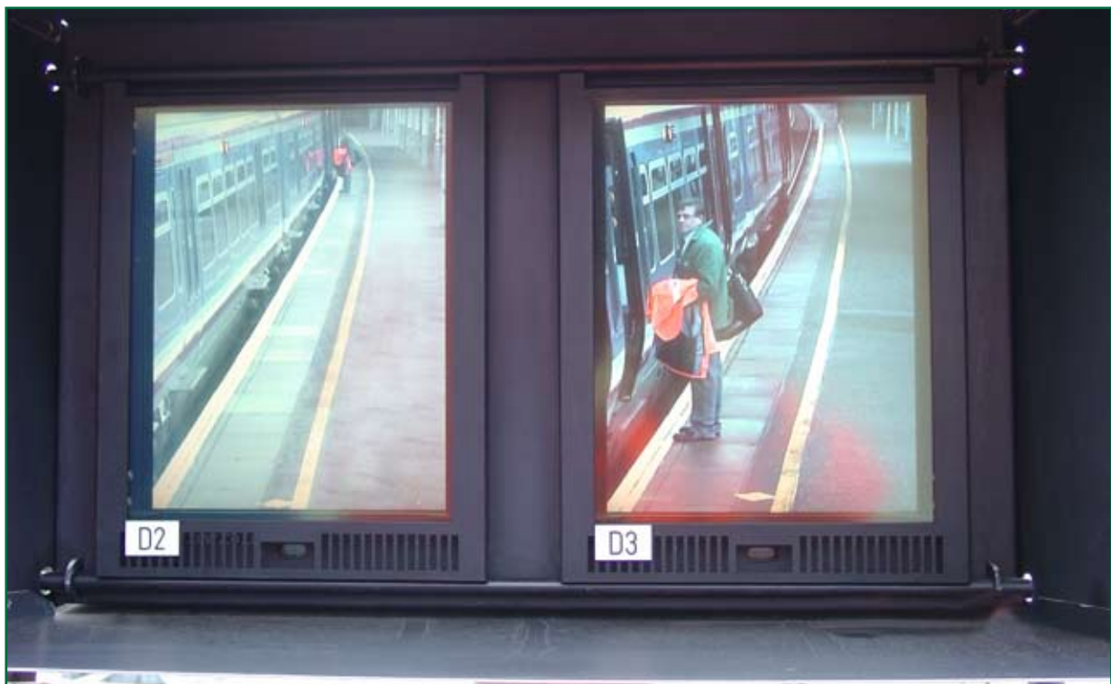
Figure 17: View from four-car monitors with a person stood at the incident door
