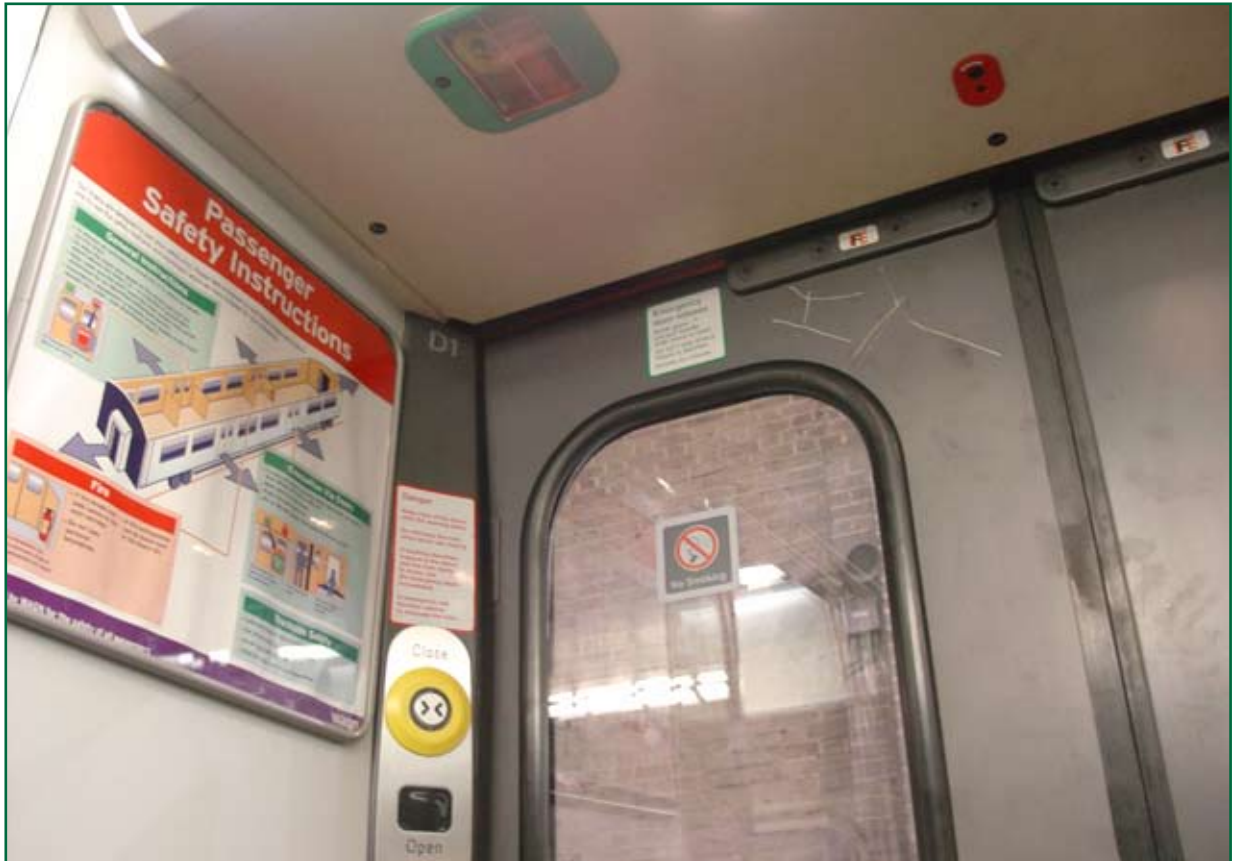
Figure 25: Signage left-hand side of the Class 365 Unit door
