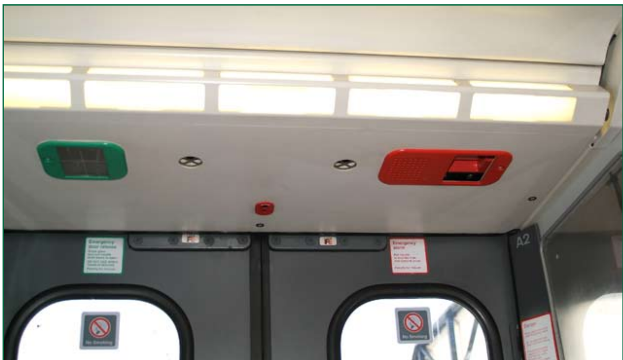
Figure 28: Door release and emergency controls over the Class 365 Unit door
