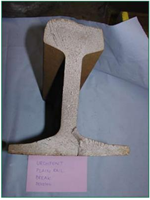
Figure 6: Broken left-hand rail from Urchfont
