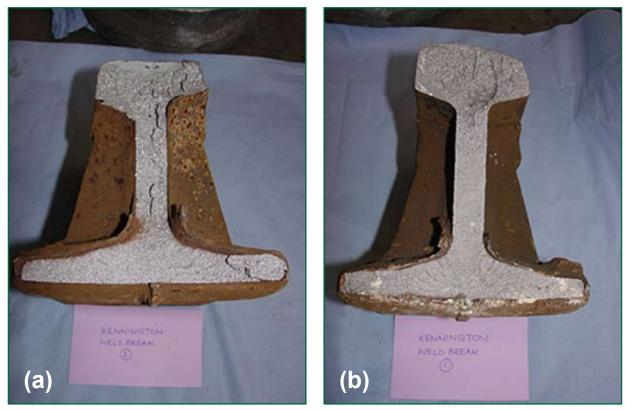
Figure 7: Broken left (a) and right (b) rails from Kennington
