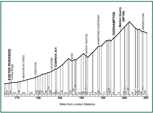
Figure 4: Gradient profile between Meldon Quarry and Exeter.
