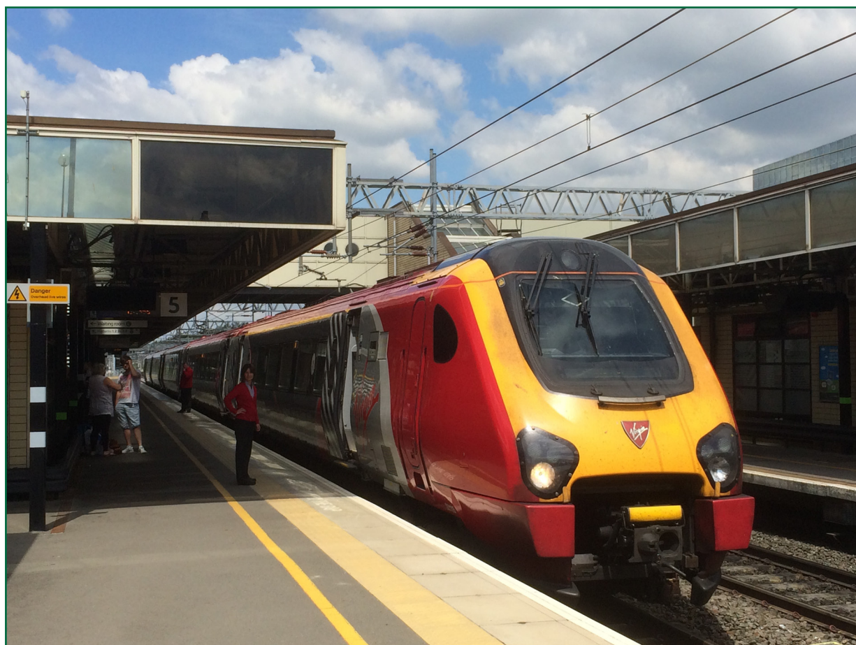
Figure 4: Class 221 diesel electric multiple unit
