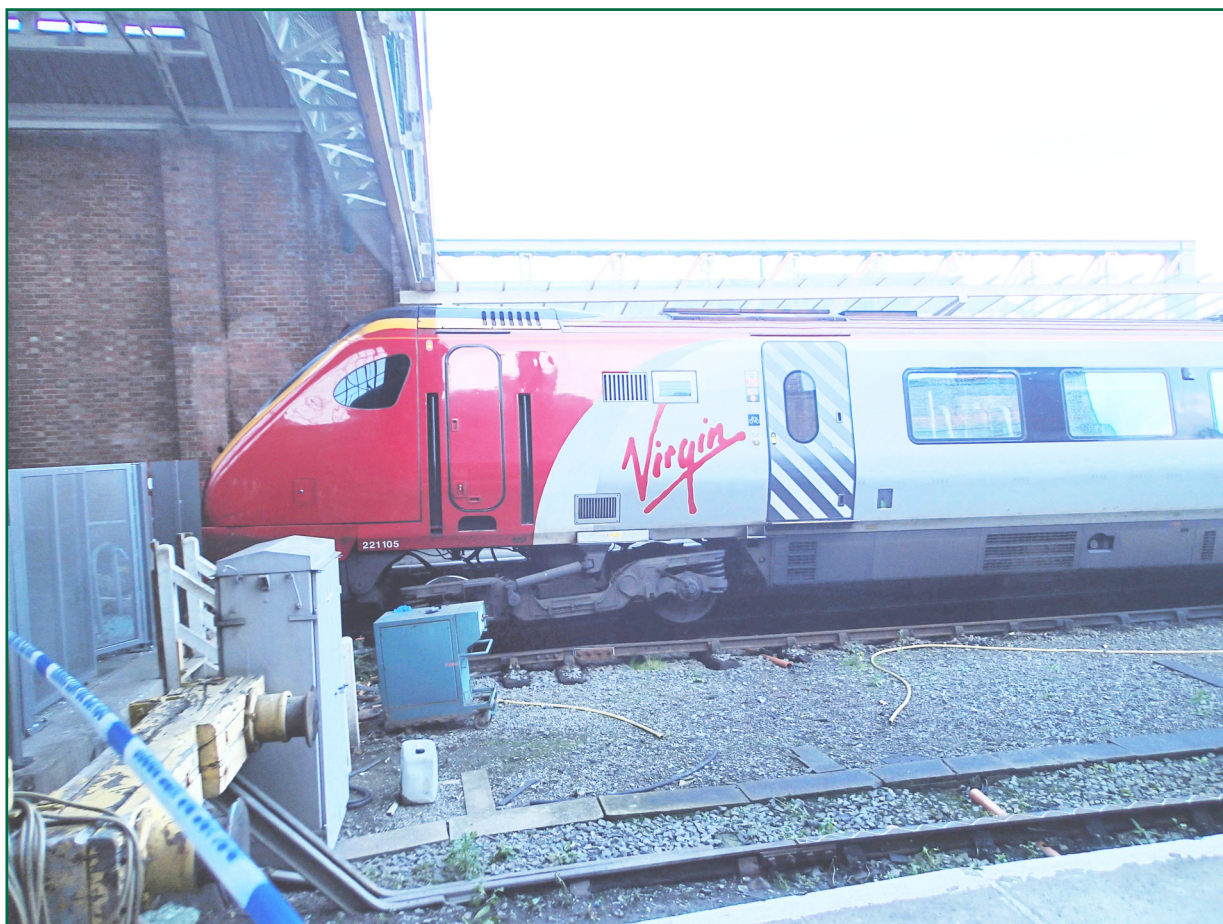
Figure 7: Front of train resting on platform showing derailed bogie
