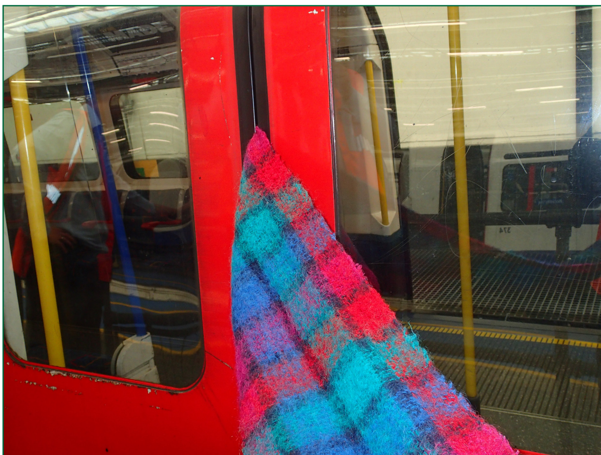
Figure 5: scarf during tests at Northfields depot
