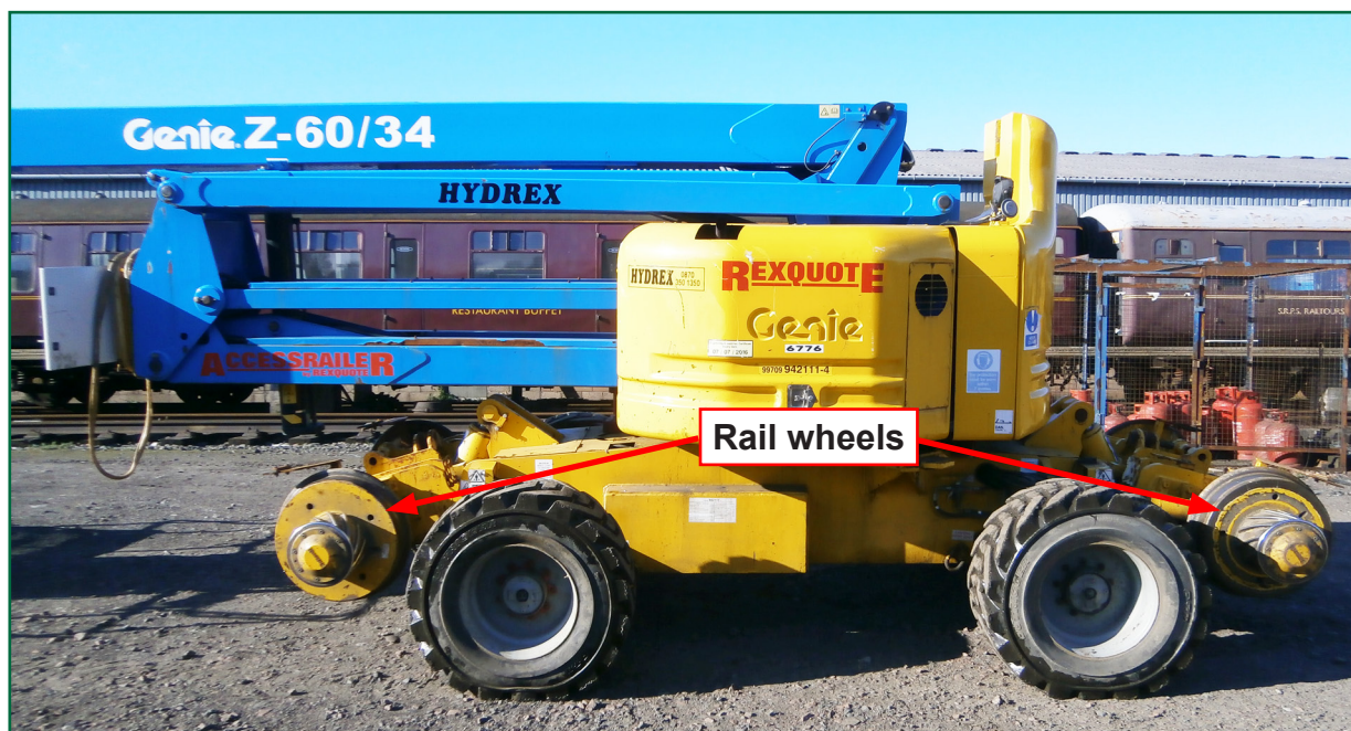
Figure 6: RRV showing rail wheel mechanisms raised
