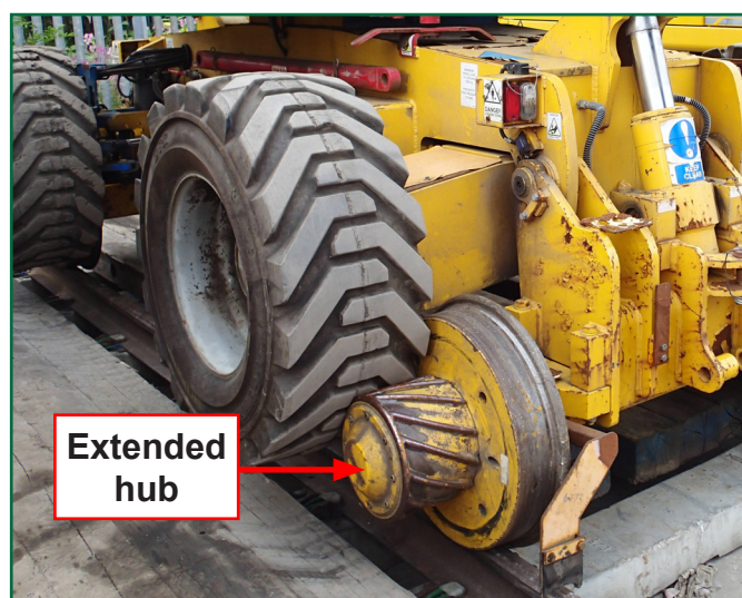
Figure 7: Rail wheel mechanism when deployed, showing contact between road wheel and rail wheel extended hub
