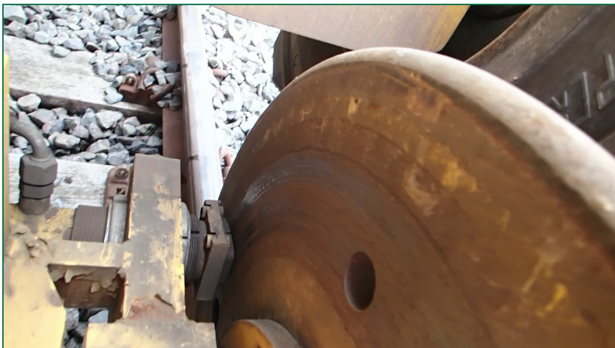
Figure 16: Surface rust present on wheel photographed during testing
