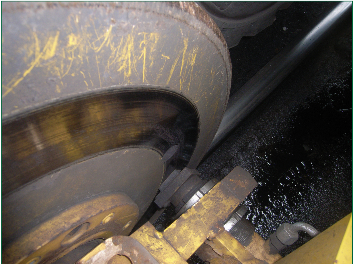
Figure 18: Clean (reflective) brake contact surface immediately after runaway
