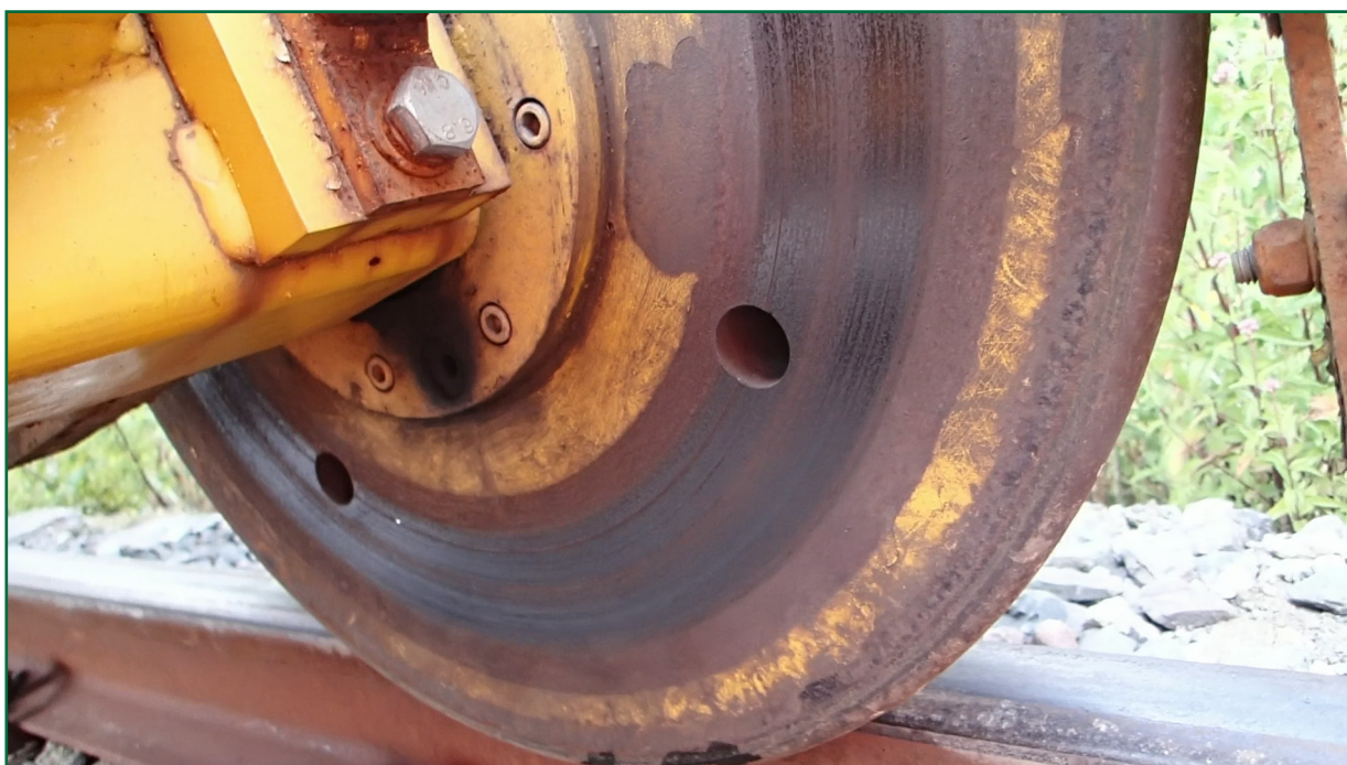
Figure 17: Typical in-service wheel contamination present photographed during testing
