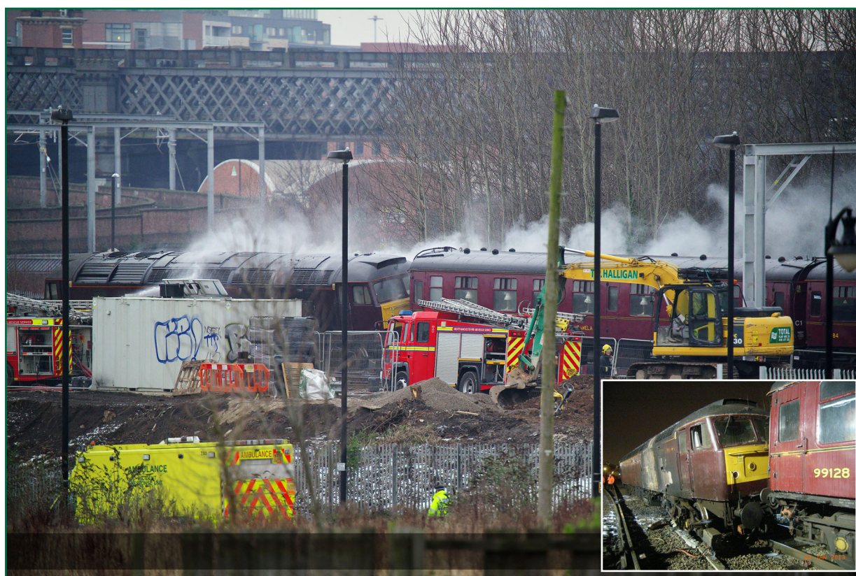
Figure 5: Derailed locomotive (main photograph courtesy of Greater Manchester Fire and Rescue Service)
