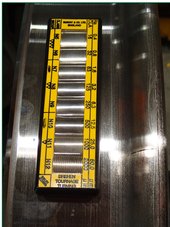
Figure 13: Surface finish sample gauge against a typical newly-reprofiled wheel
