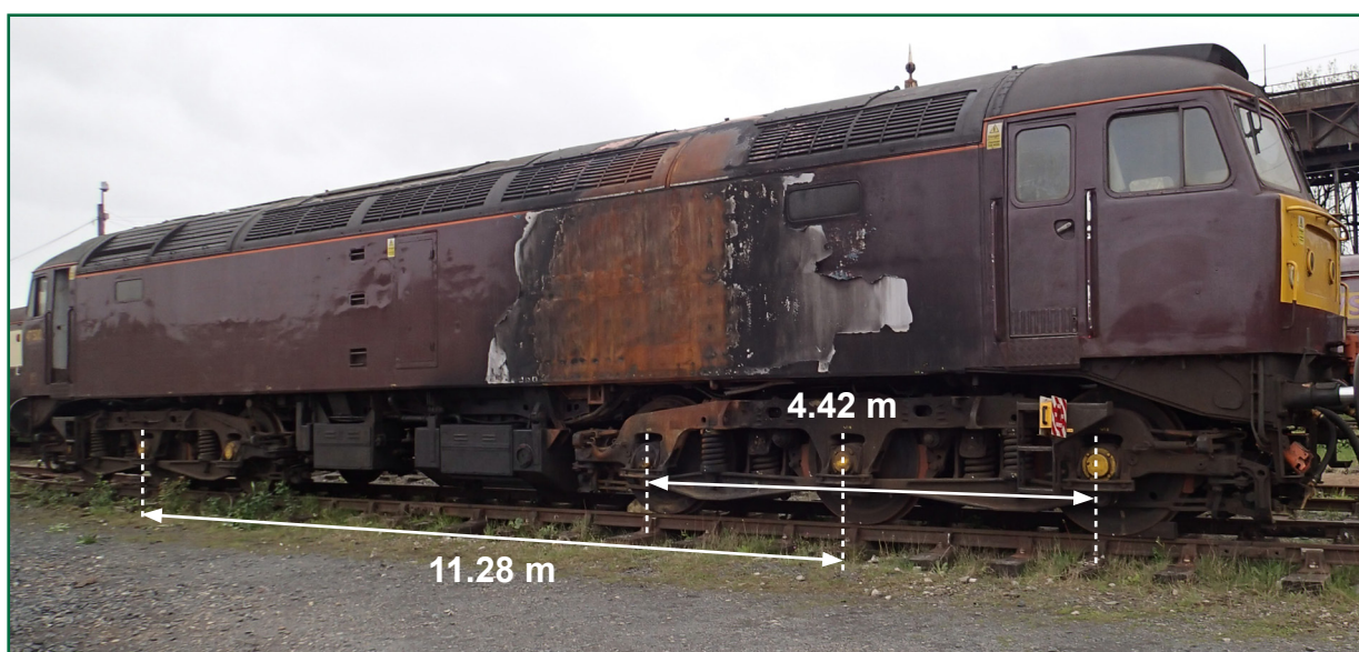
Figure 3: Locomotive 47500 showing wheelbase and bogie spacing dimensions
