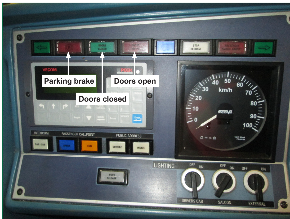
Figure 4: Driver's cab panel showing door indicator lights for closed (green) and open (red)
