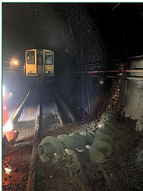
Figure 6: Auger sections and debris on the track (photograph courtesy of Network Rail)
