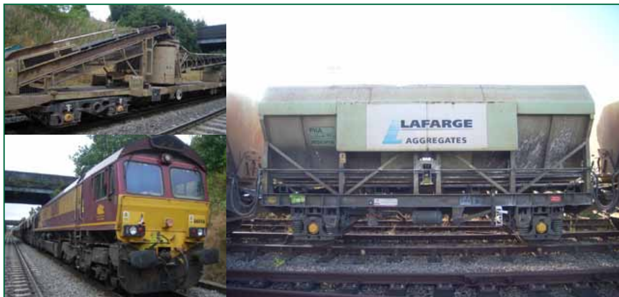
Figure 5: Train 6Z31 showing a PHA wagon (right), a KJA wagon (top left) and the locomotive (bottom left)
