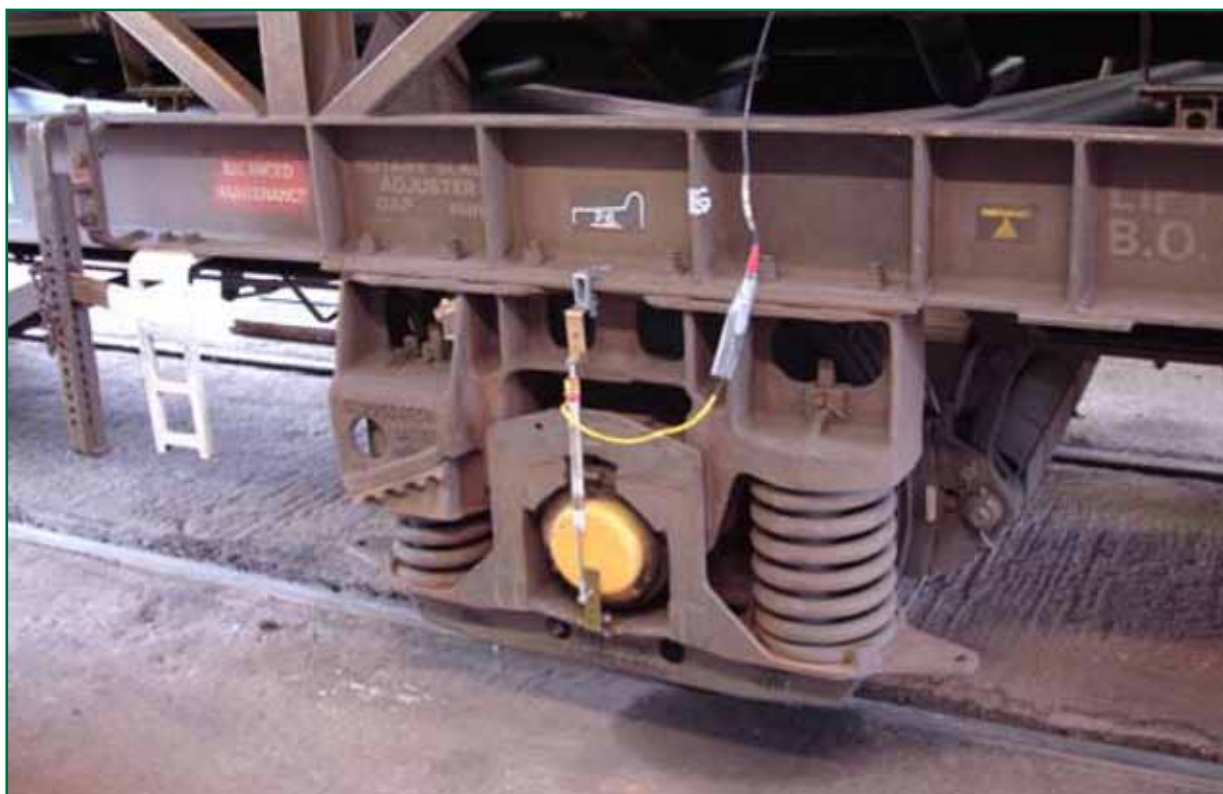
Figure 14: Instrumentation fitted to the PHA wagons that were tested (image courtesy of Serco)
