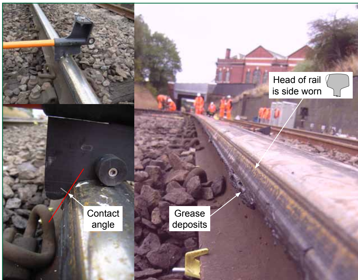
Figure 20: Side worn rail and contact angle between the rail and the wheel
