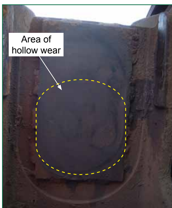
Figure 23: Hollow wear on the saddle friction liner plate on the leading left-hand corner
