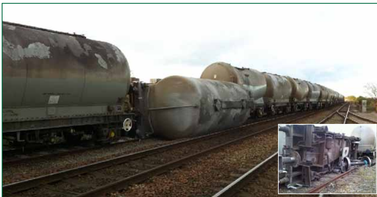
Figure 22: Train 6B32 derailed on exit to Craiginches Yard, Aberdeen (images courtesy of Network Rail)
