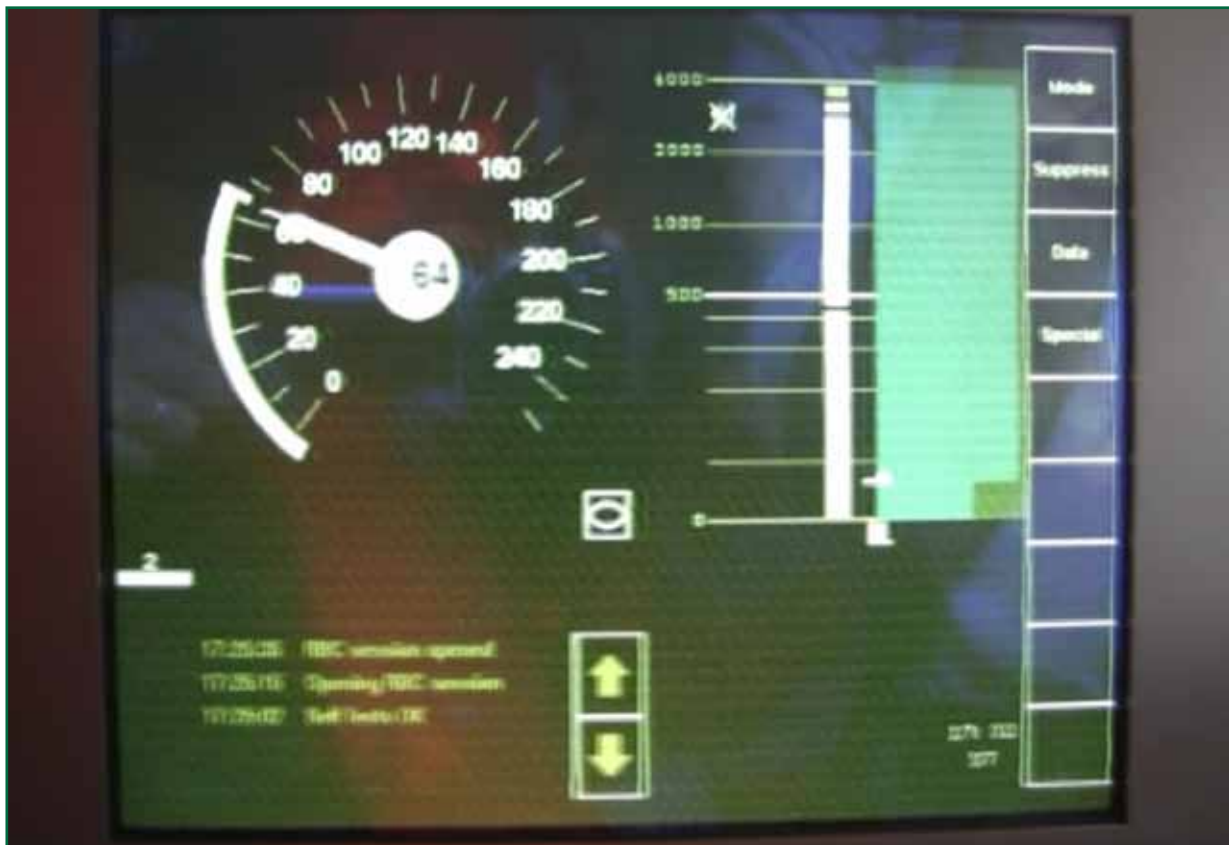
Figure 11: ERTMS DMI screen showing movement authority and speedometer needle and speed hook. Note: the speedometer is showing 64 km/h and the speed hook (maximum speed) is indicating 65 km/h
