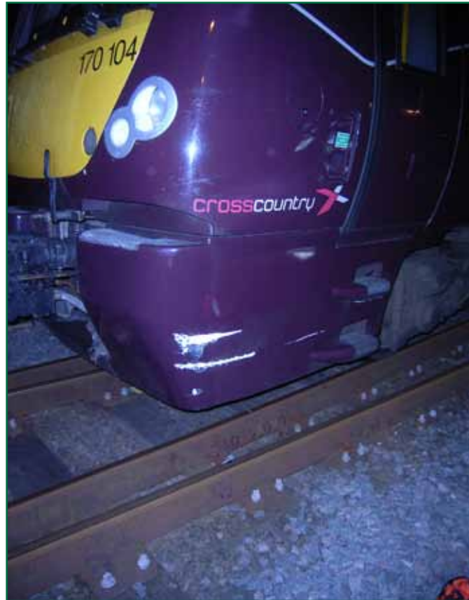
Figure 3: Damage to the front of the train
